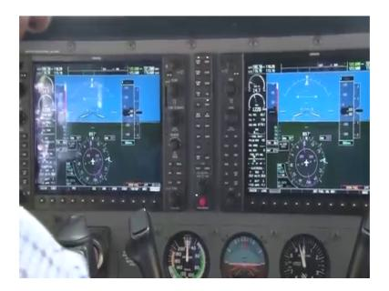
See with the engine on, now the engine is on the engine is on very first thing you have to watch for when you switch on the engine is the oil pressure, the oil pressure is supposed to register within 30 seconds to ensure that your oil has a started flowing within the engine and proper lubrication has started taking place. This is my r p m you can watch here this r p m, I need to put the engine on 1200 r p m. So, that the wild temperature comes to the limit (Refer Time: 24:56).
