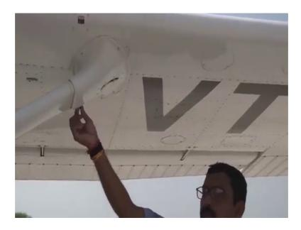
Then these are the vents, this is the vent line we ensure that the vent line this thing is not bent this is clear, there are no obstructions in this, this is about the fuel system of the aircraft now. So, this is the propeller you can see we need to ensure that the blades leading edges have no damage, the blades are the spinner is properly secured, there are no leaks in the propeller this is the oil panel, we will open this panel.
