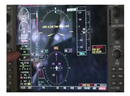
This is the normal 1000 avionics system this is my digital instrument you can see lot of parameters here on the screen manifold pressure this is the r p m this is the fuel flow this is the oil pressure oil temperature, cylinder head temperature exhaust gas temperature. Fuel quantity, left tank, right tank this is for the electrical bus voltage, battery voltage then these are the various instruments.
