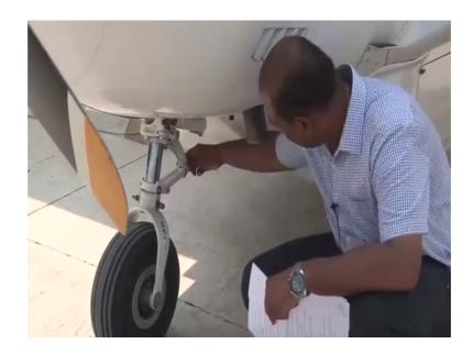
This is the nose landing gear, we need to watch for the cleanliness proper strut extension, the attachment of the talk links all the bolts are in place, all the locking mechanisms are in place and there are no leaks in the shock strut. The nose wheel we need to watch, the nose wield the proper locking is their, proper anchoring is there, there are no tire there are no cuts on the tires and proper inflation is there.
