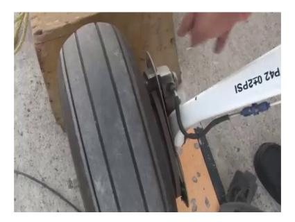
We need to see that the there are no cuts, no damage in the tire, the required creep marks are in place the required locking this, this spit pin this is properly there we need to inspect the main wheel.
