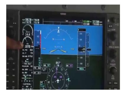
Which is the minimum r p m; that means, throttle pull out I am going to check the idle r p m that is the minimum r p m see the minimum r p m that is 600 at the moment.
