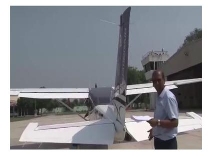
All over the area you need to see whether you are the tail plane is clean there is no damage, there is no distortion all the rivets are in place, there is no shearing of the rivet plus the elevator hinges, the hinges the bolts are in place. The movement you need to check the movement of the elevator that there is no movement, there is no binding in the movement your cables are in place, similarly in the rudder watch the hinges the bolts are in place and the movement is proper.
