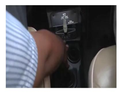
So, I have put the fuel tank selection put in the both position. So, that the fuel can simultaneously be supplied from both the tanks, this is your throttle control this is your mixture control, sorry propeller control and this is your mixture control.
