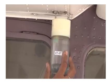
From the first point we have ensured we want to ensure that the fuel is free of dirt, there are no sediments this is another point this was the real point, this is the forward point of the fuel tank. So, we want to ensure by taking the sample from different points that the fuel is almost free of dirt, there are no sediments and the fuel is safe for use, this is a forward fuel drainage point this is the gascolator point we this is the lowest point in the fuel system.
