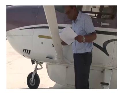
The lift struts for damaged straightness and security of attachment, these are the lift struts we need to check whether there is no damage, here they are securely attached both sides you can see one side bottom and at the top similarly on the right side also, we need to check the aileron hinges and excessive play for corrosion and security. So, these are the aileron, you can see we need to check these ailerons their movement.
