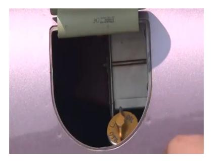
We need to see you can see the oil dipstick here, the oil tank cap we will open this oil tank cap and ensure that the oil quantity is sufficient, you can see this is the oil dipstick you can see the oil, we will wash we will clean this lipstick with a clean cloth and we will dip it again and find out the quantity of oil in the oil tank, you.
