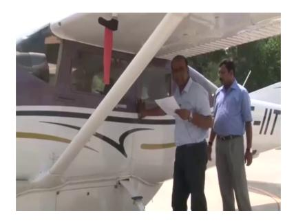
So, we need to see the skin, the aircraft skin all over for the cleanliness for any damage for any scratches or something, rivets you can see the rivets here we need to watch the rivets whether the rivets are there some rivet has not sheared off. So, all over the fuselage we need to inspect this thing check for security and operation of door and their latches check condition and the hinges.
