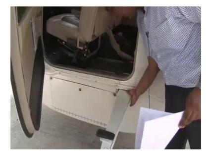
We need to watch do a visual inspection, weather all the things are in place whether there is no crack, the main and nose wheel tires for creep marks general condition and correct inflation you can see this is the main wheel.
