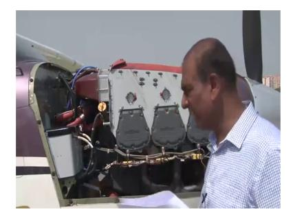
Now, coming to the engine this is the right side of the engine 3 cylinders, we see whether all the screws they are in place there are no leaks, there are no leaks all the fuel lines they are in place the spark plugs are properly anchored. So, now, the cowlings have been opened this is Lycoming IO 540 engine on the Cessna 2 0 6 aircraft, it is a 6 cylinder engine we are on the right side these are 3 cylinders, first second and third cylinder.
