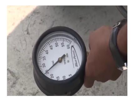
So, this is a tire pressure gauge we call it a t p g, it is properly calibrated we need to have a calibration ted, this calibration also has got a validity. Before using this instrument we
