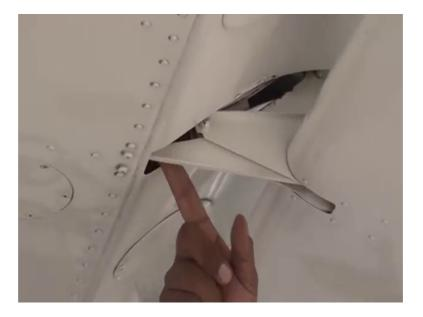
The flap track we need to see the weather the track has not worn off the rollers are in place. So, all the tracks and the rollers have to be inspected on both sides, on the left side and as well as the right side.
