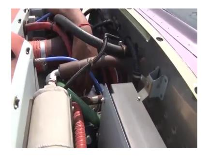
This is the oil cooler, then you have the magnetos here you need to ensure that all the electrical connections in the magnetos they are in place they are properly secured. So, after doing a complete visual inspection of the entire engine we will put back the cowlings and we will do a engine ground on.
