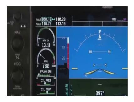
So, you have seen all along your parameters are in green range, to cut off the engine to switch off the engine I will pull this lever the mixture control out which will stop the supply of fuel to the engine and it and the engine will eventually shut down. You can see I am pulling this lever out the fuel supply is shut and the engine has stuck, the engine is out now I put the ignition switch back to off.
