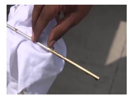
So, you can see here this is the maximum mark and it is slightly less than the maximum mark which is 11 quarts the oil in the tank at present is sufficient for a safe flight.
