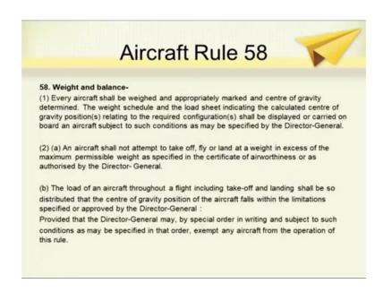
Aircraft Rule 58 is for weight and balance. So, every aircraft shall be weighed and appropriately marked and center of gravity determined. The weight schedule and a load sheet indicating the calculated center of gravity position, relating to the required configuration shall be displayed or carried on board an aircraft, subject to such conditions as may be specified by the Director General.
