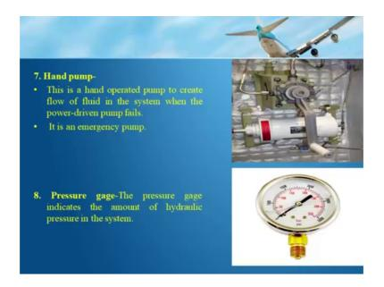
Now, next is the hand pump, we have seen in case of an emergency this is an emergency pump. This is a hand operated pump which is used to create flow of fluid in the system when the power driven pump fails.
