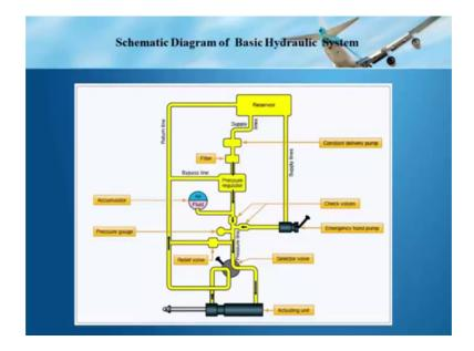
Now, coming to a basic hydraulic system. So, you can see a basic diagram of the hydraulic system, there are various components fitted in this system this is the reservoir here you have the pump, this is the filter, pressure regulator, accumulator, these are the check valves, this is the hand pump, here is the pressure gauge, this is the relief valve, this is the selector valve and this is the actuating unit.
