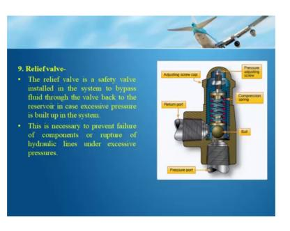
Then we come to the relief valve the relief valve it is called as a safety valve, which is installed in the system to bypass fluid through the valve back to the reservoir in case excessive pressure is built up in the system.
