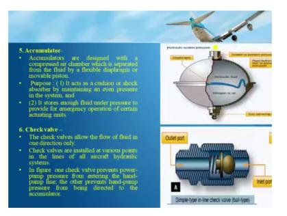
Coming to accumulator accumulators are designed with a compressed air chamber, which is separated from the fluid by a flexible diaphragm or movable piston. It is purpose is to act as a cushion or shock absorber by maintaining an even pressure in the system.
