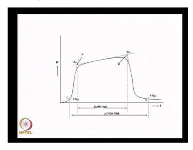
We talked in terms of burn time. Two tangents intersecting; this is shown for progressive case: A to B is the burn time. The time of one- tenth of the pressure at ignition to one-tenth of this pressure at burn out over here, is what is the action time. Well these are all about the solid propellant rockets.
