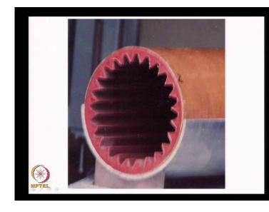
See this is how pyrogen propellant grain looks. It is like a solid propellant rocket only you do not need to generate thrust. We provide a multi point star shown in red. When the propellant here is ignited, it generates hot gases that ignite the main motor.
