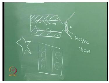
Since we need to build pressure in the port volume, we put something like a closure at the nozzle. When pressure builds up and the motor is ignited, the closure is thrown out. We make sure that after adequate pressure is generated around 5 bar to 6 bar, the closure is dislodged. This closure is known as a nozzle closure.
