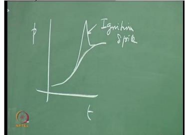
And this erosion effect, because it increases the burn rate can also lead to the ignition spike since at this time the port volume is small and velocities would be large. The larger mass burning rates could provide the spike.
