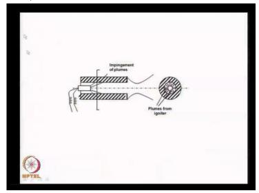
This is an igniter may be a pyrotechnic igniter. It produces these plumes which impinges on the propellant surface, ignites the surface also pressurizes the cavity. These are the individual plumes, which are igniting the surface. The flame spreads and then the gases move out through the nozzle and this is how ignition takes place.
