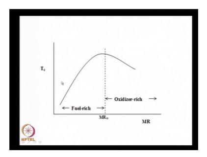
The temperature of the gases as a function of mixture ratio is such that the maximum temperature occurs just below the stoichiometric. We had a slight shift; instead of maximum temperature occurring at stoichiometric it occurs at slightly fuel-rich conditions. But when we need a much lower temperature maybe we have to operate the gas generator in a very fuel-rich region such that we get only around 800 to 900 K i.e., a very oxidizer-rich region wherein I get a low temperature.
