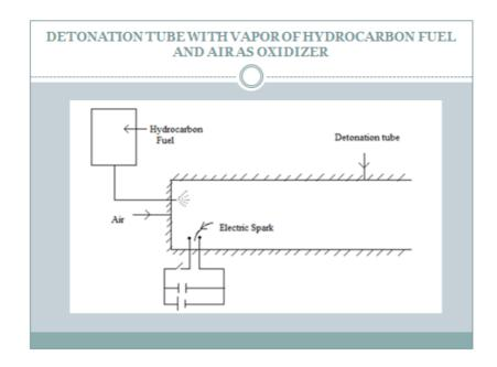
The detonation tubes used in practice are a few centimeters in diameter. The maximum frequency at which a single detonation tube can be fired is a few tens of cycles per second. This depends on the time required for filling the tube with the mixture, the travel of the flame and detonation in the tube and the time taken for purging the tube of the combustion products. If a number of the detonation tubes can be clustered together as
