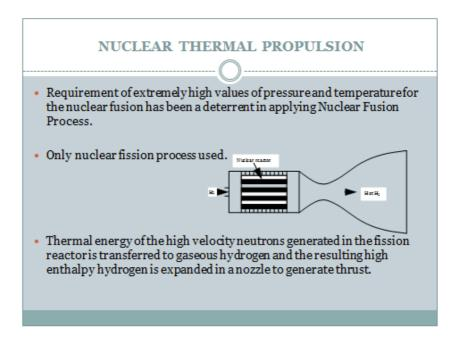
When the thermal energy of the fission process is directly used, as illustrated in this slide, we call it as nuclear thermal propulsion (NTR). It is also possible to convert the nuclear energy into electrical power and use the electrical power in electrostatic and electromagnetic rockets. The use of electrical power from nuclear reactions for propulsion is spoken of as nuclear electric propulsion (NEP).
