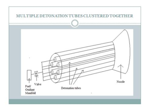
shown in the slide, the number of pulses of thrust generated per unit time can be significantly increased. This is done by operating the tubes successively one after the other. A common mixture preparation chamber feeds the different tubes. However, each of the tubes has its own ignition source. With a large number of detonation tubes, the thrust generated becomes almost continuous rather than being in discrete pulses. A divergent nozzle is provided to enhance the thrust.
