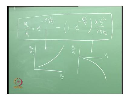
As  $M_u/M_i = e^{-\Delta V/VJ}$  and  $M_P = M_i - M_f$  when divided by  $M_i = M_f/M_i$ . We substitute  $M_f/M_i$  =  $e^{-\Delta V/VJ}$  and we get  $(1-e^{-\Delta V/VJ})\chi V_J^2/2\eta t_b$ . Hence the expression for the useful mass.
