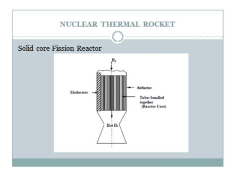
The fission of uranium is initiated by sending in neutrons from an auxiliary chamber. The core, as shown, is surrounded by moderators and reflectors to control the rate of generation of the neutrons. Hydrogen gas is admitted through holes in the reactor and it gets heated by impact with the neutrons. Since the residence time of hydrogen in the reactor is not significant, the efficiency of heating is not high.
