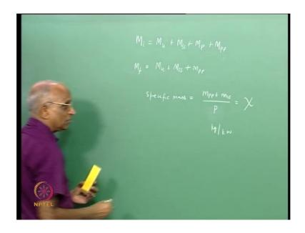
Now, if I have a battery; it is going to be heavy. That means in addition to the usual structural mass in a chemical rocket, there are other mass which are to be included in the initial mass of hardware. Let us go back to the Tsialkowsky's equation or the rocket equation.
