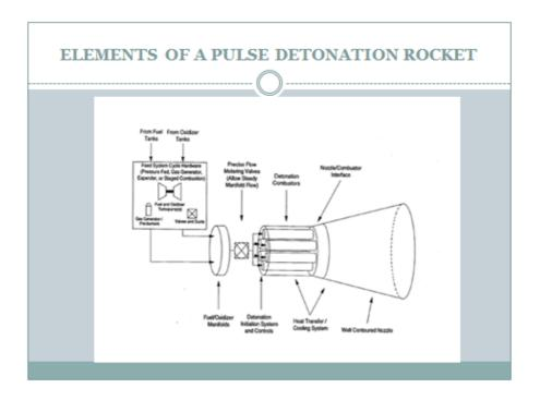
The elements of the pulse detonation engine comprise of propellant tanks, inlet valves, detonation tubes with electric spark system and blockages in the tube for transition of the flame formed by the spark to a detonation. The construction is simple. However, the
