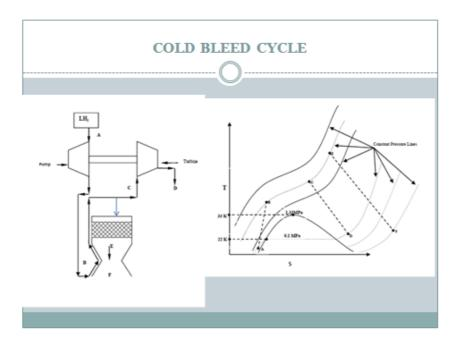
There are different versions of the feed cycle such as a cold bleed cycle in which the cold hydrogen is injected into the chamber and the exhaust from the turbine is let out through an auxiliary nozzle. It is similar to a gas generator cycle. It is also possible to have a hot bleed cycle in which the hot gases from the chamber are bled and mixed with cold hydrogen to drive the turbine.
