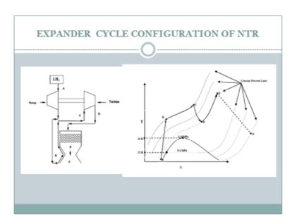
The jet velocity  $V_J$  is given by root of two into specific enthalpy drop from E to F.
