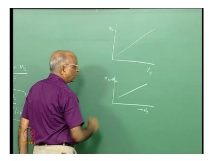
I say, well the payload mass, the useful mass  $M_U$  is a function of  $V_J$ . If I look at  $V_J$  alone may be as  $V_J$  increases, the useful payload will go up. This is because we have a higher jet velocity. But, a higher jet velocity results in a higher power and therefore, the power that means the values of  $M_{PP}$  plus  $M_S$  also increases as  $V_J$  increases.
