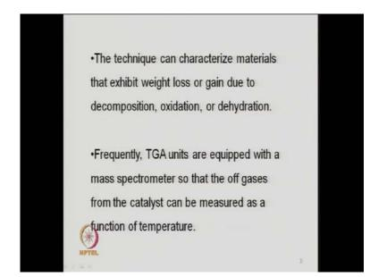
So, the technique, this can characterize materials, which is weight loss or gain, because sometime if you have a recursal of the metal and then, you have the oxidation or oxidizing environment, it may oxidize also, during heat treatment, you can have the weight gain also. So, weight gain. So, depending upon, that you can find out that delta H, which is related to temperature for a given weight gain. So, you can find out the enthalpy of the reaction also.
