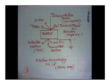
So, this is I will take little later not for this but, generally for a primary electron beam or x rays, the principle is similar the x ray has the wavelength of 100 angstrom of the order of that. So, it means, it will cover a wider surface something like that but, when the electron beam if you see, it has the wavelength, which is less than one angstrom. So, it can give you the atomic information.
