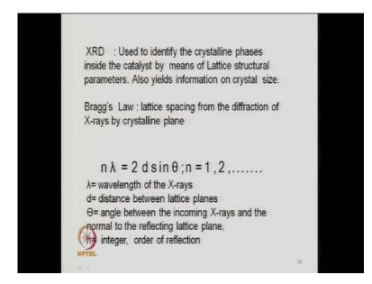
So, this is written here, this x-ray diffraction pattern used to identify the crystalline phases, inside the catalyst by means of lattice structural parameter. So, the arrangement of the atoms on the metals, how they are arranged and when you have the x-ray beam and that reflects. So, there can be different kind of x-ray sources, which of different energy beam energy and then, you see that what angle there is diffraction.
