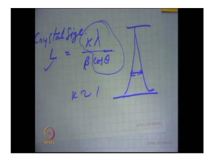
So, crystal size which is sometime represented by l is equal to k lambda over beta cos of theta something likes this. So, this is the constant, all this k is roughly 1, it is a property basically 1. So, beta is the peak of half height. So, it means if at a given angle of diffraction 2 theta, this is the total height. So, this is something like here, beta is the peak width of half height and radian units.
