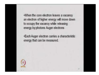
But now, it is not the primary core electron but, a secondary electron so, this is what the structure here it is shown that the electron release from the top layer. So, this is the top layer this is your inner surface and electron beam which is here and you can measure the energy of these secondary electrons now not the core electron. So, the electron which is released from the top layers so, their energy can be measured.
