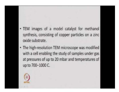
So, just what is here the TEM image of a model catalyst for methanol synthesis consisting of copper particles on a zinc oxide substrate, that another example which are shown taken and high resolution transmission electron microscope was modified with cell enabling. This study of sample under gas at pressure up to 20 million bar and temperature up to 700 and 1000 2000 degree centigrade.
