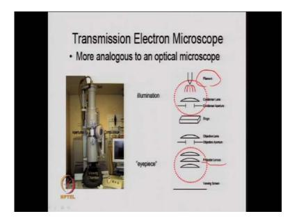
So, the idea is again that it is a high energy beam a kind of energy beam basically but, high energy electrons in one electron and so, you have a filament a if you take this is a filament here and just these are the condenser lens to have the monochromatic relights. So, energy source so and this is your objective lens here objective aperture and this is your viewing screen.
