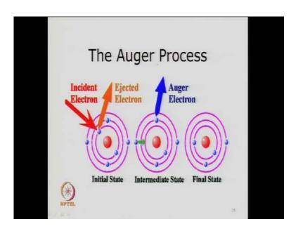
So that, is what the auger process we have discussed is that the auger electron this is what the core electron something like here. So, the incident electron ejected this is the secondary electron so and the vacancy creates this going into the inner core. So that, is the final state now when the electron has left the process. So, you can get the information in the similar way you can get the intensity as a function of kinetic energy.
