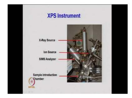
So, of a unit and 1 of the units so, x-ray source the ion source then secondary and mass spectrometer Analyzer then sample introduction chamber and then the other side detector source.
