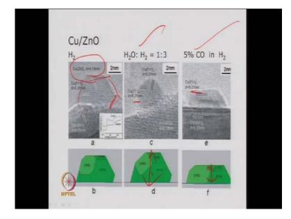
So, this is just a experimental data we just indicate that what information you can get from the transmission electron micrograph. So, you can see here that this because, of the edges the shape can be seen here, this is what the shape of a metal copper on zinc oxide. So, this is what so and that has been pictured here and this way you can see the edges. Now, here because, the different edge there will be diffraction from the edges.
