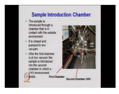
So, this is just a kind of induction chamber if you look at here the actual picture of XPS so, that what the how the samples are introduced, the sample is introduced.
