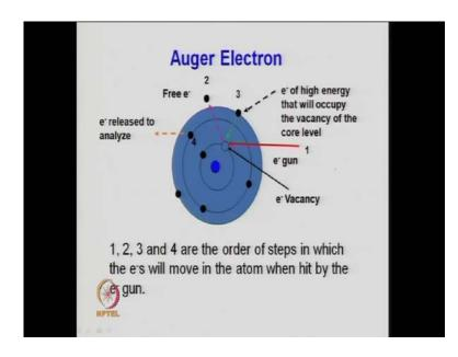
So this is your core, so electron gun comes to the core here and then the vacancy comes from here and since so, this is your step number 1 this electron will go out because, energy try to go out rather and once this goes the form here, the electron of high energy that will occupy the vacancy of core level because, this is now vacant. So, electron will come out from here and then since there again the electron from this outer one will again release and this will go out.
