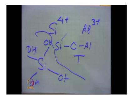
So, when I say zeolite it means the silica s i 4 plus and a 1 3 plus now they so are connected and they are connected to the oxygen bridge. So, you will have a structure something like say s i o a l like this and then when I just look at s i it has like this O H O H O H so on O H. So, you have a structure like this a tetrahedron form because just like if you look at a methane molecule the hydrogen is attached to the carbon, which is at the center.
