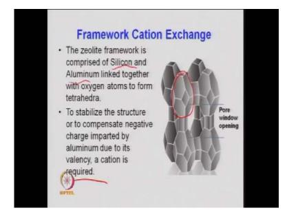
Then a framework of cation exchange does the same thing .What I talked is that it is comprised of a silicon, and aluminum link together with oxygen atoms. Which forms a tetrahedral, which is shown before also?
