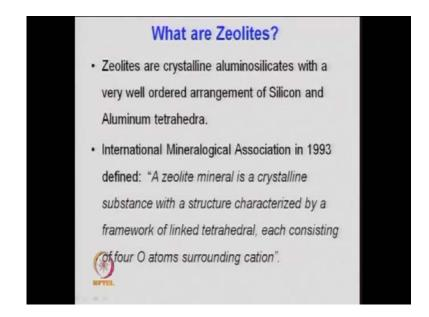
So, as I told that we look at a crystalline material in terms of catalytic activity. So, degree of crystanality becomes important and that will depend on the frame work and the structure the of that zeolite cage. So, it is not a definite pore opening, when you look at a
