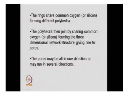
So, rings share common oxygen or silicon forming different polyhedral, now the depending upon the oxygen connected to the ring. As I said it may be 4 member it maybe 6 member 5 member, 8, 10, 12, different oxygen member rings zeolites are available larger the number of rings, the opening will be wider it will be wider. So, modernite, like that hozashied different kind of zeolites is available depending upon these rings.
