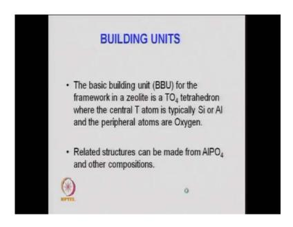
So, the basic building unit for the framework of zeolite, which we call T O 4 silicon a tetrahedron, where the central t atom maybe silicon. It can be aluminum and the peripheral atoms are oxygen. So that is what I discussed.
