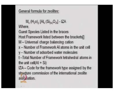
So, basically if you look at the zeolite formula. It depends on different compositions of aluminum and the silicon atom in the group. So, clay material also has something like this the calcium aluminite it's again a clay material calcium oxide and aluminum oxide site or Caroline, this porcelain material ceramic material. It can also have these kinds of the silicon and aluminum but, there is not a definite kind of structure.
