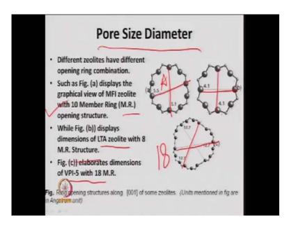
You have the different kind of frameworks, so opening of zeolites. So, generally when you define, you will sometimes you say average diameter pore diameter, but, all the time. When you talk zeolite catalyst? You define it to a into b, so it has 2 type of opening like you see here 5. 5 versus 5. 5, both this is same on both sides, which is the cage opening of that.
