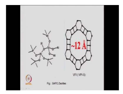
So, this is again a type of SAPO zeolite, where the origin of petroleum institute and this is a 12 angstrom and that is the pore opening of the zeolite and number of rings can be calculated 1 2 3 4 5 6 something like that so, different kind of silico alumino phosphate
