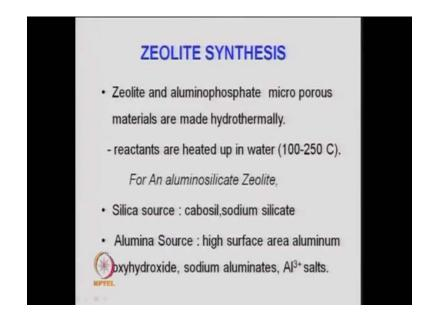
So, with this background let us, come to the synthesis because, once you look at this kind of definite structure definite pore opening a definite silicon to alumino ratio so, the preparation becomes very crucial part in the zeolite synthesis, unlike you are the non zeolite materials or other catalytic material like silica alumina or seria zirconia so, these type the weather preparations are well known or well defined in terms of either watt impregnations co precipitations solder methods.
