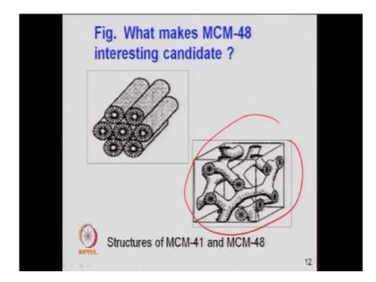
So, they have certain importance like this MCM 48 you see it is a 3 d type of structure and this is just an MCM 41 which has just a laminar or 2 d or laminar structure,1 d different kind of channels can be here.
