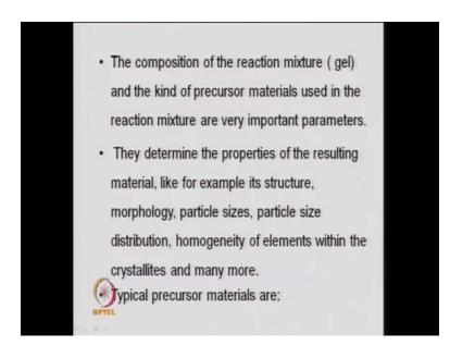
So, the composition of reaction mixture that is gel and the kind of precursor material used in the reaction mixture, they are very important as I said for the zeolite synthesis they determine the property of the material for simple morphology particle size distribution, homogeneity. So, all these will depend on the type of the raw material so, these are all I have discussed basically.
