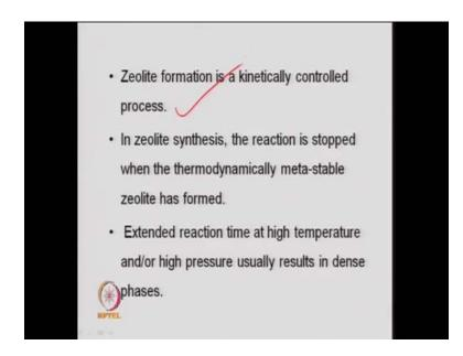
When slow reaction zeolite synthesis, the reaction is stopped, when thermodynamically Meta stable zeolite has formed. So that, is just from the thermodynamics so, you have to give enough time the reaction is kinetically controlled and based on that you have to just identify whether 24 hour or 7 days, sometime 20 days so, because the reaction or the kind of silicate to Aluminate framework which is forming depending upon the raw material.
