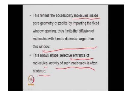
So, because of this 3 d it refines the accessibility of molecules, what I was talking the safe selectivity so, they are safe selective so, accessibility of the molecules inside the pore geometry of the zeolite by imparting the fixed window opening so, they have very definite window size and thus limits the diffusion of molecule within kinetic diameter larger than this window.
