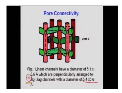
So, this is what the frame work has been shown here so, horizontal and the vertical so, the channels roughly if you look at here, the linear channels have diameter of 5.1 by 5.6.
