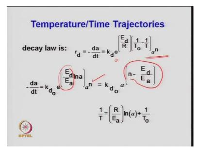
So or in one way you can say substitute the value of 1 upon T minus 1 upon T0 that is equal to R upon Ea ln of a from this equation the value is substituted here. So, 1 upon T0 minus 1 by T and that has been changed to R upon. So, which is cancels now because this R that R gets canceled. So, finally you have minus E d upon Ea and Ea upon Ed upon Ea ln of a so that can be written in terms of the power form. So, kd0 a to the power n minus Ed upon Ea we get.
