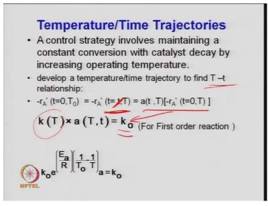
So, one can write this because K you know from Arrhenius law equation K0 E to the power minus E upon RT that is Arrhenius law equation. But, when I am writing k1 by k2 so that is represent this is the now rate constant measured at temperature t0. So this is rate constant measured at temperature t 0 times E to the power e upon r1 by t0 minus 1 by T. And, that is equated to the initial rate that is when the temperature is t0.
