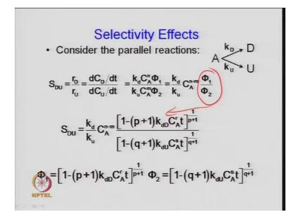
S o, SDU is equal to rD upon rU which is written in terms of these two rates and can be recohilated with the kD times CA to the power n which I have already talked. And, that can be now substituted because this ratio is known now. So, this is just a substitution of this term here, So, how the selectivity change? Because, of the deactivation will depend on the orders of each that is the first one towards d and the second one towards q or U. And, also the concentration of
