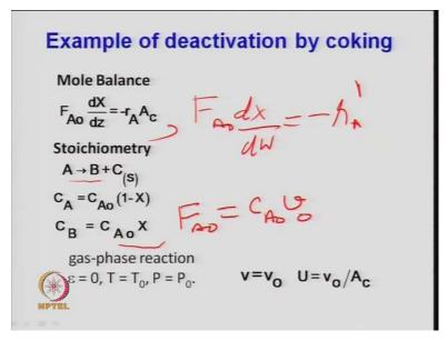
So, if you look at this rate equation this is your design equation or one can write as I said in the form of FA naught dx by dw is equal to minus rA dash for the catalytic reaction generally we use this. But, wd is the mass of the catalyst which will depend on the density of the catalyst in the bed row B times this volume dv. So, dv is a C times dz. So, one can write the expression in either form v is constant volume system volumetric feed rate.
