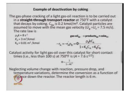
So, this is just as Example for practice so here if you look at the problem is something like that a gas is cracking of light gas oil is carried out in a straight through transport reactors.
