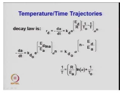
So, this your dk law so your rate of deactivation or the rate for the deactivation is related to the activity. So, rd is minus da by d T that is equal to kd times again it is related with the Arrhenius constant. So, kd is at refresh temperature that is measured at temperature T0 times E to the power minus EdE to the power Ed upon r now times one by T0 minus 1 by T and, times a to the power of n.
