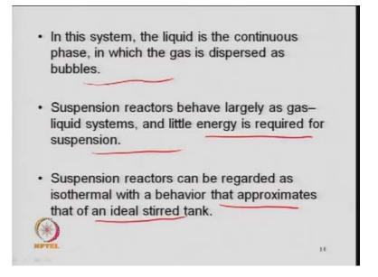
Some advantage if you will look at here in this system, the liquid is in continuous phase, in which the gas is dispersed as bubble. So, gas bubbles are coming from the bottom and liquid is already present along with the solid, so liquid is in continuous phase and gas is being dispersed in a form of bubble. So, even a small size particles, gas bubbles, so now you need to design a better spurger so that, the bubble size should be controlled, otherwise the mass transfer resistance will be an issue.
