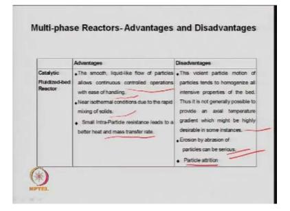
So, it has again some advantage, but simultaneously some disadvantage, so one thing is that, smooth liquid like flow , because it is a fluidized bed, so you just the particles are flowing just like a fluid. Only thing that you need to have some high fluid rate or superficial gas velocity, all these hydrodynamic studies need to be done in order to make the bed or particle fluidized at all the time. So, this allow a continuous control operation with ease of handling.
