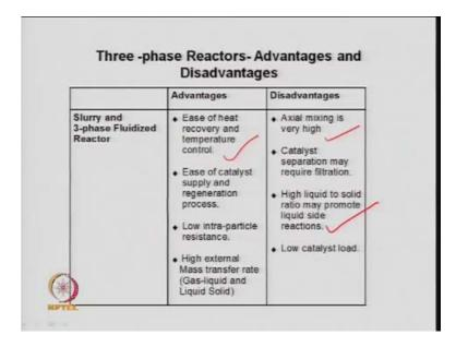
Then, again a slurry three phase fluidized reactor, so here again we have some advantage and disadvantage, so just I have tabulated them. So, slurry three phase fluidized bed reactor ease of heat recovery and temperature control, because you have a in the slurry phase, so particles are fine. So, as in the fluidized bed reactor, you know whatever the advantage, these will be here also, so ease of recovery and heat and temperature control is one.
