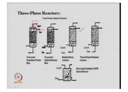
Three phase system is more complicated, so I will just discuss this part today, here you can see that, you have a solid inside the reactor, back. And then, that flow can be concurrent or counter current, so that also it depends on the concentration, difference which is required or the kind of the contact between gas liquid and solid, which is desired. So, both type of combination may be used, so here you can see the liquid comes from the top, so we need a distributor here.
