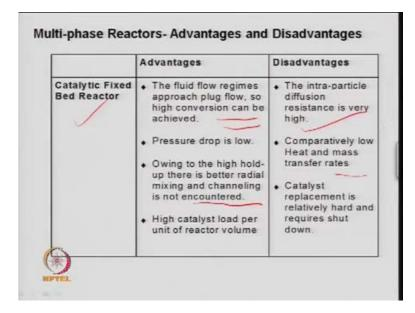
But, if you look at the compression, a catalytic fixed bed reactor just and a multi phase reactor, so catalytic fixed bed reactor it has some advantage, but disadvantage also. So, these kind of reactor system will have some advantage and some disadvantage also, one has to do all these exercise in order to find like dust reactor for the given process in the presence of the catalyst. So, here the catalytic fixed bed reactor, the fluid flow region approaches to the plug flow.
