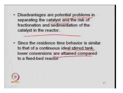
Because, this is what the separation of the catalyst, you have fine powder, smaller particle size, so separation of the catalyst and the risk of fractionation and sedimentation of the catalyst in the reactor. If the stirrer is not well designed or if the dusty of the catalyst is high then, there may be the chance that, some of the catalyst will get sedimented or some of the catalyst may, if it is very fine, it may get out along with the liquid.
