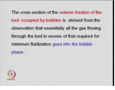
So, cross section from bubble to emulsion – transport; the cross section of the volume fraction of the bed occupied by the bubbles is derived from the observation that, essentially, all gases flowing through the bed in excess of that required for the minimum fluidization goes into the bubble phase. So, basically, what you get? That you get from the minimum fluidization condition. So, gas flowing through the bed, which is in excess is nothing but what goes to the bubble phase.
