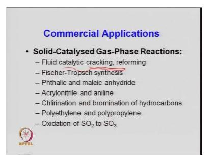
But, fluidized bed reactor as I said, they are widely used. So, one is the solid-catalyzed gas-phase reaction; they are widely used. So, one of the most important is the FCC cracking. So, more than 420 FCC reactors are available worldwide and they are
