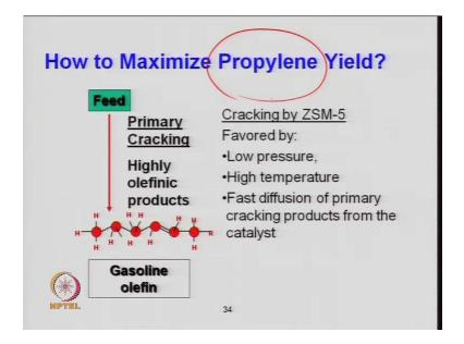
Propylene is nowadays in the refinery and petrochemical. The high yield of propylene is desired. So, how to improve the propylene unit? So, selective catalysts are required; which can maximize the olefins, especially the propylene. And, that is generally for the petrochemical purpose. So, when you have a pyrolysis type process, where the
