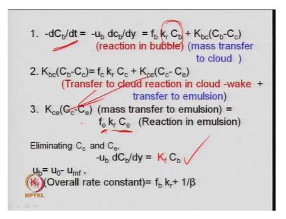
So, you can very easily write down the rate of disappearance of b; which you write minus d C b by d t; that is, change in concentration of b with respect to time rate. And, you know now that, f a naught d x a is equal to minus r a. And, that is here mentioned in terms of this convective term, which is f a z, which is loss; and between f a at y, which is written in terms of C a into u times e. So, basically, it is a mole balance.
