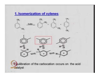
So, these are some reactions, which are generally shown in the isomerization. And, one can look at and depending upon the catalyst, which is used, one can have the process.
