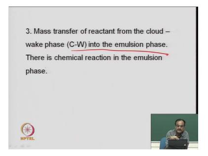
And then third step – when it reaches to the cloud and wake, there is no mass transfer; mainly, it is a chemical reaction. So, that is basically in the emulsion phase. So, mass transfer of reactant from cloud-wake phase to the emulsion phase – that we already talked. And now, there is a chemical reaction in the emulsion phase; and there is no further transfer.
