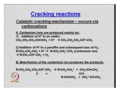
Similarly, cracking reaction; and where the again the larger molecular weight compounds are cracked into smaller. And, again zeolite or silica alumina type catalysts are used in this process.
