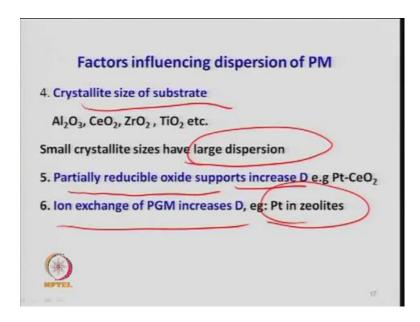
So, sometimes you reduce it to a size of the say 50 micron or say just 100 nanometer where you find powder, the idea is that the one thing in that you are increasing the surface area of those particles. Because, small and second thing that the particles when you have a smaller they can bind, because see the particles property change, when you change the particle size and when you go to the nano level.
