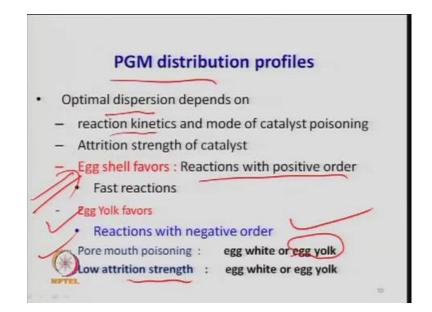
So, the distribution profile for this platinum group metal, if you look at the optimal dispersion depends on the kinetics of the reaction and mode of catalyst poison. So, the poison pick that is a especially, when you have a naphtha or hydro carbon fraction which
