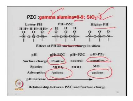
So, this I have shown here if you look at here, that for your example for gamma alumina the PZC is between 8 and 9, and if you look at silica then it is 3, so it means for gamma alumina at 8 or 9, there is no charge on the surface, when you have taken the pH 8 or 9. Same thing for silica a pH is 3 the surface has no charge, but if you look at here for the silica we have taken the different case, so this is at lower ph, at lower pH the surface will have a positive charge.
