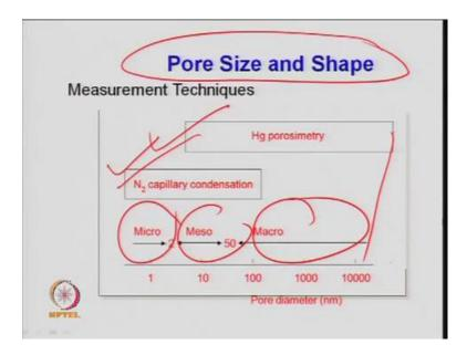
So, If you look at the pore size, shape distribution of the pore, they are very important and need to be determine. So, we have several methods by which we can determine the pore size and shape of a catalyst, which are based on physical adsorption reaction, so one of the most important or commonly known is known as mercury porosimetry method. The second one is known as nitrogen adsorption desorption method capillary condensation, that is phenomenon which is based on capillary condensation.
