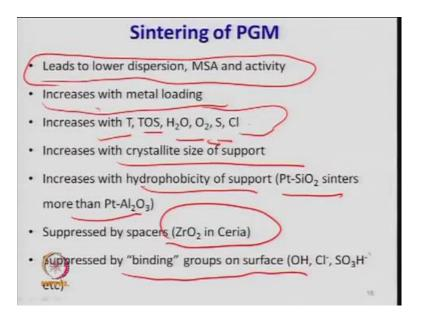
Sintering, so that is what you get during firing of a catalyst, so calcination, so it leads to a lower dispersion, so metal surface area and activity drops, so MSA refers to metal
