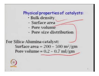
If you look at the characterization of the catalyst or a physiochemical properties of the catalyst, which are generally produced or developed during the catalyst preparation. So, this is also very important issue that, bulk density, that density of the pallet, density of the powered particle, density of the powdered material and when you made a tablet from that then, what is the density.
