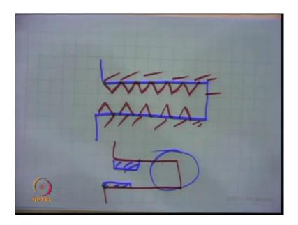
So, this what I mean to say that rate of drying can give you a pores material, where the metal may be deposited uniformly like this in the pore, so this is one pore in a solid like this, there are millions of the pores. So, active metal is deposited like this on the surface, the second case may be it is deposited just on the outer periphery, say only this surface is covered, at low drying rate and then it is extreme everything may go on this side at the pore head.
