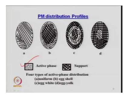
And this example which I have correlated here earlier in terms of the egg shell or egg yolk, so similar thing that this precious metal or platinum metal distribution profiles has been shown a typical profile. So, these dots represents the active phase and this is representing the support, cross or this shaded silent lines or the support power pore. So, you can see here that we were talked 4 type of active phase distribution, so uniform type, so everything is distributed uniformly on the surface.
