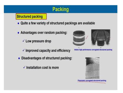
So, structured packing we have quite a few varieties of structured packing are available, one of them is the interlocks high performance corrugated structured packing you can see how it is designed and has very high surface area then flexeramic corrugated structured packing made as no ceramic materials and also it is a structured packing.
