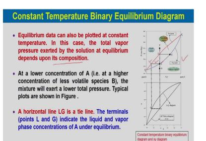
Now, we will discuss about the constant temperature binary equilibrium diagram. Equilibrium data can also be plotted at constant temperature. In this case the total pressure exerted by the solution at equilibrium depend upon its composition. So, a lower concentration of A that is at a higher concentration of less volatile species B, the mixture will exert a lower total pressure typical plots are shown in this figure. So, over here, so this is Pxy diagram at constant temperature.
