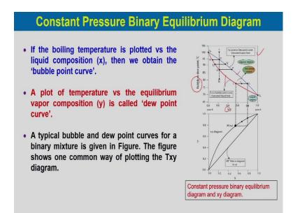
So, first we will consider constant pressure binary equilibrium diagram. So, if the boiling point temperature is plotted versus the liquid composition x, then we obtained the bubble point curve. So, in the top figure over here you can see, if we plot x versus bubble point, so then we can obtain the bubble point curve. So, this is Tx the bottom curve red line over here, this one is the Tx or bubble point curve or saturated liquid line.
