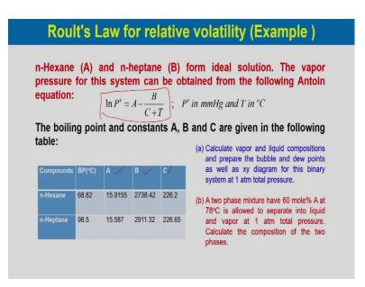
So, now let us take an example for using the Raoults law for relative volatility to solve the problem n-Hexane which is considered component A and n-Heptane considered component B from the ideal solution. The vapor pressure for this system can be obtained from the Antoin equation. this is the Antoin equation ln P V is equal to A minus B by C plus T and P V is in millimeter Hg and P is in degree centigrade.
