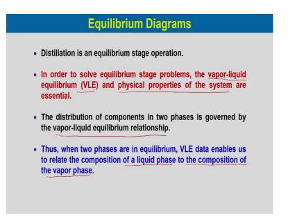
Now, distillation is an equilibrium stage operation. So, as you can see if there is an intimate contact between the gas and liquid and each tray and we consider it is it reaches the equilibrium between the liquid and vapor. So, distillation is considered is an equilibrium stage operation. So, in order to solve the equilibrium stage problems, the vapor liquid equilibrium and physical properties of the systems are essential.
