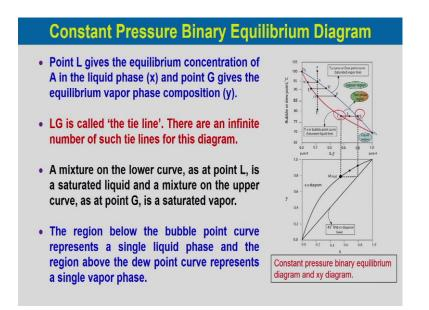
Point L gives the equilibrium concentration of A over here you can see at any point at L gives the equilibrium concentration of A in the liquid phase x and point G gives the equilibrium vapor composition y. If we just join these two points L and G is called the tie line. We can draw infinite number of such tie lines for this diagram; Txy diagram. A mixture on the lower curve at point L, at this one is a saturated liquid and a mixture on the upper curve that is at point G is saturated vapor.
