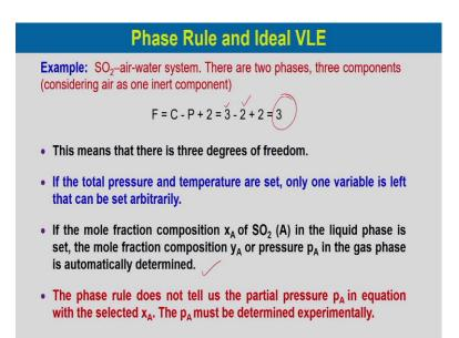
Now, consider an example sulphur dioxide air water system. So, we can see that there are two phases. One is the gas phase which will have sulphur dioxide in air and in the liquid phase which is water three components sulphur dioxide and water and then we can consider air as a single component considering an inert, no component or assuming an inert component.
