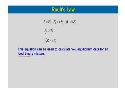
So, we can write the total pressure is equal to the partial pressure of A plus partial pressure of B. Now if we just add them x P A V plus 1 minus x P B V, then we will have P A star by P t would be equal to x, P A V by P T and hence, we can write y A star P t would be equal to x P A V. So, the Raoults law equation can be used to calculate the vapor liquid equilibrium data for ideal binary mixture. So, please remember that, this is only applicable for ideal binary mixture.
