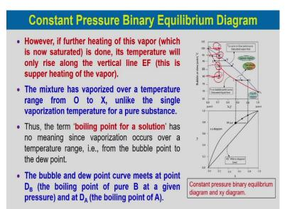
If we further heat, this vapor which is now saturated vapor at this location, if we further heat its temperature will only rise along the vertical line EF. So, from these E, it will vertically go to F.
