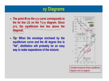
The point M, you can see over here which is xy point on the x y curve correspond to the tie line LG. So, this is L and this is G and this point M is called the tie line which is corresponding to the LG line. Since y greater than x, the equilibrium line lies above the diagonal. Because, diagonal x is equal to y, if y is greater than x then it will lie above the diagonal line; so, it is above the diagonal equilibrium line so, this is the equilibrium line.
