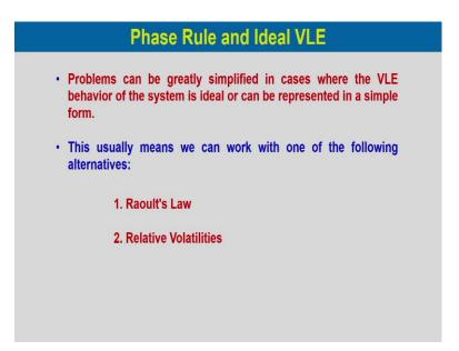
Now, this problem can be greatly simplified in cases where the VLE behaviour of the system is ideal or can be represented in a simple form like, this is usually no means we can work with one of the following alternatives that is, either we can use Raoult's law or we can use Relative Volatility. So, either of these two can work to simplify solving these problems.
