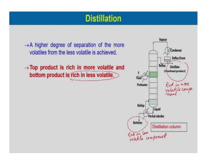
And the vapors which goes up it will increase the more volatile component. So, a higher degree of separation of the more volatile from the less volatile is achieved in this way. So, top product what we will get over here in the distillate is a more volatile component and the bottom product will be rich in less volatile component.
