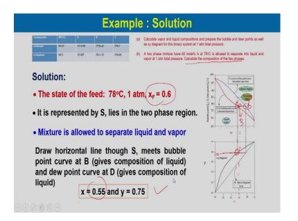
Now the second problem is a two phased mixture having 60 mole percent of A at 78 degree centigrade is allowed to separate into liquid and vapor at one atmosphere total pressure.
