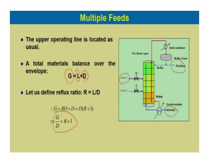
The upper operating line is located as usual, a total material balance over the envelope if we do. So, distillate which flow at the top of the column is G that is the gas inlet at the bottom of the tower and liquid which is coming out at the bottom and then the distillate which is going out at the top.
