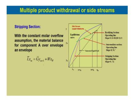
Now, if you consider stripping section with constant molar overflow assumption the material balance for component A over envelope know over an envelope we can write L bar into x m would be equal to G bar y m plus 1 plus W x W.
