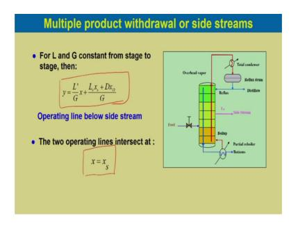
Now, this we can rearrange and we can write y n plus 1 would be equal to L n by G n plus 1 into x n plus L s x s plus D x D by G n plus 1. For L and G constant from stage to stage then we can write y would be equal to L dash by G into x plus L s into x s plus D into x D y G.
