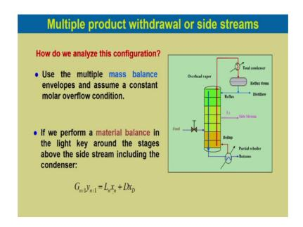
How do we analyze this configuration? Use the multiple mass balance envelops and assume a constant molar overflow condition. If we perform a material balance in light
