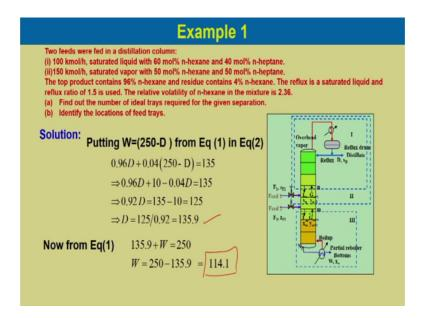
So, from this know putting the values in equation know 2. So, we can obtain so, distillate is 135.9 kilomole per hour and similarly, W would be 114 kilomole per hour. So, we can calculate know by doing the material balance species mole balance and the overall material balance, we can calculate the distillate and bottom flow rate.
