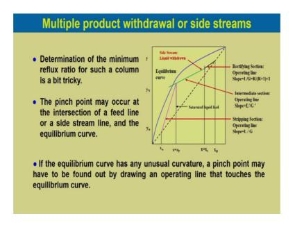
So, determination of the minimum reflux ratio for such a column is a bit tricky in this case, the pinch point may occur at the intersections of a feed or a side stream line and the equilibrium curve.
