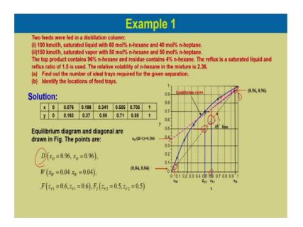
Now, equilibrium data that relative volatility equation is given. So, equilibrium data we can calculate and we can thought the equilibrium diagram which is shown over here in the blue line.
