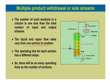
The number of such sections in a column each one less than the total number of input and output streams. The liquid and vapor flow rates vary from one section to the other section because you have intermediate product withdrawal.
