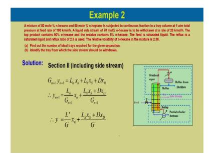
Now, section II including the side streams the material balance equation would be y n plus 1 would be equal to L n by G n plus 1 into x n plus L s x s plus D into x D by G n plus 1.
