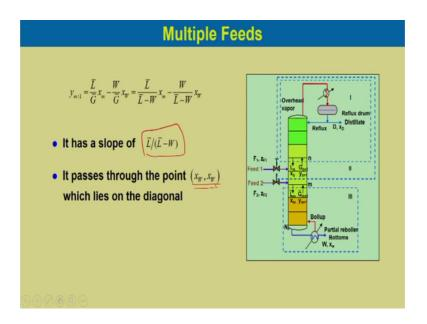
Now, it has a slope of L bar by L bar minus W slope of the operating line section and it passes through the point x W x W which lies on the diagonal.
