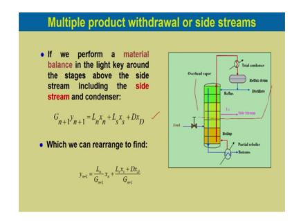
If we perform a material balance in the light key around the stages above the side stream including the side steam and condenser, we can write G n plus 1 into y n plus 1 would be equal to L n x n plus L s x s plus D x D. So, this is including the side stream; so, envelope over here above this.
