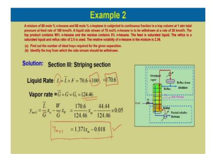
Now, for section III which is know stripping section the liquid rate L is equal to L bar plus F. So, L bar is know 70.6 plus know feed is 100 kilo mol per hour. So, it would be 170.6 that is kilomol per hour is the liquid rate. The gas vapor rate remains know constant for this section as well it is G bar would be equal to G would be equal to G 1 which is 124.46.
