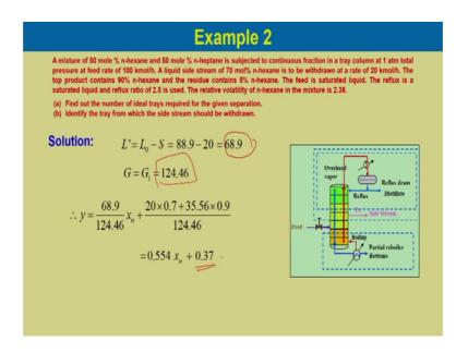
If we substitute the values L dash would be equal to L naught minus S. So, which is 68.9 kilomol per hour G would be equal to G 1. So, it is 124.46. So, operating line equation y would be equal to 0.554 x n plus 0.37.
