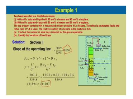
So, slope of the operating line would be 0.894 in this section II.
