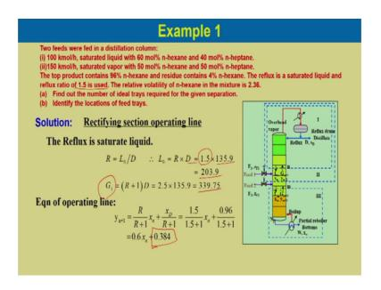
So, now we can know plot the know we can find out the rectifying section operating line, the reflux is saturated liquid. So, R would be L naught by D. So, which is L naught would be equal to R into D, the reflux ratio is 1.5 which is given over here. So, if we put 1.5 into distillate is 135.9. So, it is L naught would be equal to 203.9. So, the G 1 which is know vapor flows from the top tray is R plus 1 into D which is 2.5 into 135.9 so 339.75.
