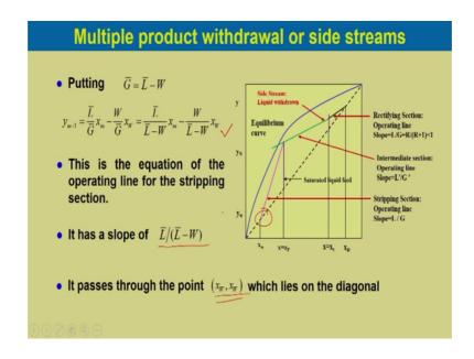
So, this is the stripping section operating line equation and it has slope L bar by L bar minus W as usual, it passes through the point x W, x W and it lies on the diagonal.
