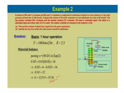
And though putting the total material balance over here. So, we can get distillate is about know 35.56 kilo mol per hour. So, this is distillate. And similarly know we can calculate the bottom product which is 80 minus D which is equal to know 80 minus 35.36 which is 44.44.
