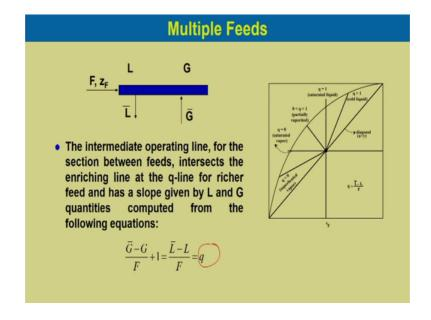
So, you can see know if we do the balanced equation for feed line. So, this is F z F would be equal to know which is entering into the feed L is the top column know, liquid flow and now from the top of the section and know from the top of the section and know from feed tray it is L bar and going into the feed know feed tray is G bar and going out from the feed tray is G.
