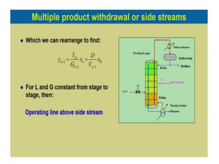
And from here we can write know y n plus 1 would be equal to L n by G n plus 1 into x n plus D by V n plus 1 into x D. For L and G constant from stage to stage, then operating line above the side stream.
