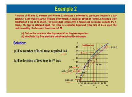
So, we know the composition over here in the rectifying section is 0.9,  $0.9 \times (())$ ,  $\times D$  and we know over here 0.05, 0.05 in the stripping section.
