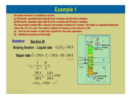
And for section III, the liquid rate would be L into know section II the liquid rate in the section II. So, which is 303.9 and vapor rate because feed is saturated vapor. So, it would be 339.8 minus F 2. So, it would be 339.8 minus 150. So, which is 189.8.
