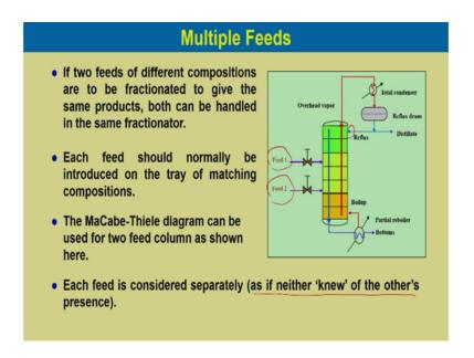
So, you can see over here in the distillation operations, we have feed 1 and feed 2. So, two different feed are given to the distillation column and we have single reflux in at the column and then as per the other design we have boiler at the bottom which have reboiler.
