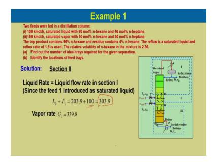
Now, for the section II liquid rate would be equal to liquid rate in the section I, because since the feed 1 introduced as a saturated liquid. So, L naught plus F 1 would be equal to 203.9 plus 100 that is the feed which is introduced. So, it is 303.9 and vapor flow is 339.8.
