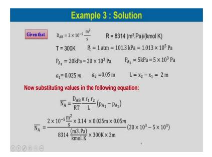
Now, if we substitute the parameters which are given D AB RT Pt and partial pressure of component a at 1 and partial pressure of component two component a at 2 and then, the other values a 1 a 2 and the length.
