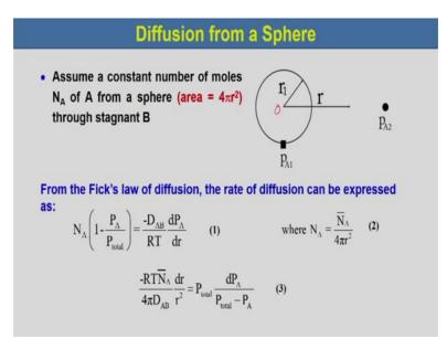
So, let us consider a sphere whose centre is O and the radius is r 1 and then, the area radius is varying with time and the partial pressure at the bulk is P A2 and at the surface of the sphere is P A1.
