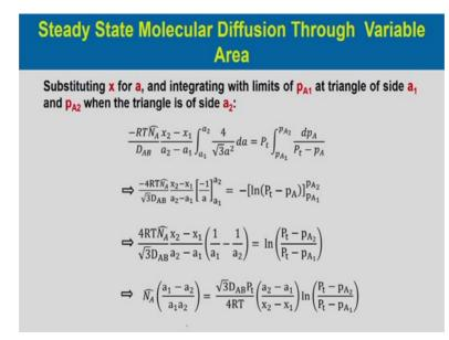
Now, if we substitute x for a and integrating with limits of partial pressure of component a at 1 at triangle of side a 1 and partial pressure of component a at point 2, that is p A2 when the triangle is at is of side a 2, we can write minus RT NA cap divided by D AB into x 2 minus x 1 by a 2 minus a 1 integral a 1 to a 2 4 divided by root 3 a square d a which would be equal to p t integral p A1 to p A2 d pA divided by P t minus p A.
