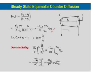
So, now let us consider C 1 is equal to r 2 minus r 1 divided by x 2 minus x 1. So, we can write the above equation as N A cap by pi integral x 1 to x 2 d x divided by C 1 x plus 1 whole square which would be equal to minus D AB by RT integral p A1 to p A2 dp A.
