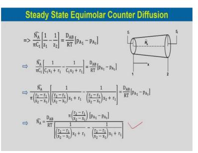
So, this would be written as N A cap by pi into C 1 whole into 1 by z 1 minus 1 by z 2 which is equal to D AB by RT into p A1 minus p A2.
