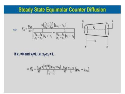
Now, after now if we put x 1 is equal to 0 and x 2 is equal to L and x, that means x 2 minus x 1 is L. The total distance from point 1 to point 2 the above equations, we can write N A cap would be equal to D AB by RT into pi r 2 minus r 1 by L into p A1 minus p A2 divided by 1 by r 2 minus 1 by r 1 which would be equal to D AB by RT into pi r 1 into r 2 by L into the partial pressure gradient p A1 minus p A2.
