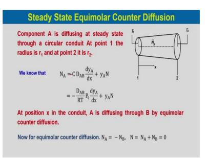
Now, let us consider steady state equimolar counter diffusion. So, this is a cylindrical geometry uniformly tapered. So, component A is diffusing at steady state through a circular conduit. At point 1 the radius is r 1 and at point 2 it is r 2.
