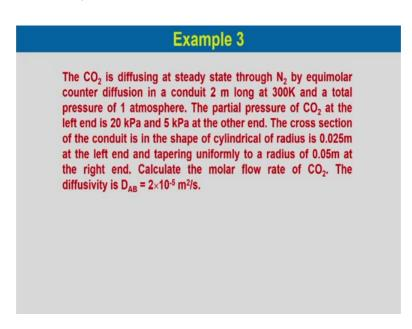
Now, let us consider one example. The carbon dioxide is diffusing at study state through nitrogen by equimolar counter diffusion in a conduit of 2 meter length at 300 Kelvin and
