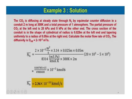
So, if you substitute these values in the following equation, you would obtain N A bar would be equal to this which would be equal to 0.00785 into 15 divided by 4988400 into 10 to the power minus 2 kilo mole per second which is equal to N A bar is equal to 2.36 into 10 to the power minus 10 kilo mole per second.
