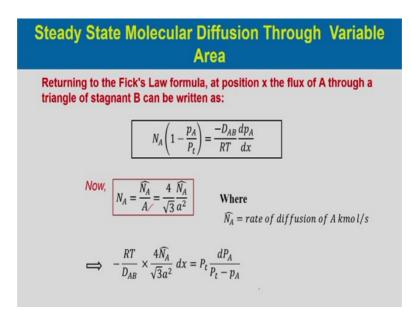
So, now returning to the Fick's law formula at position x of A through a triangle of stagnant B can be written as N A into 1 minus p A by P t is equal to minus D AB by RTdp A dx.
