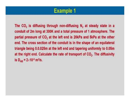
Now, let us consider one example. The carbon dioxide is diffusing through non-diffusing nitrogen at steady state in a conduit of 2 metre long at 300 Kelvin and a total pressure of 1 atmosphere. The partial pressure of carbon dioxide at the left end is 20 kilopascal and 5
