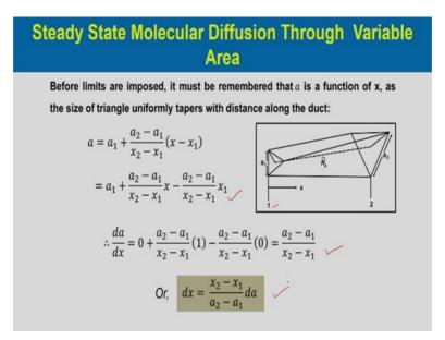
Now, before limits are imposed it must be remembered that a is a function of x. That means, a is varying with respect to the distance x as the size of the triangle uniformly tapered with distance along the duct. So, we need to have a relation between a and x. Now, a would be equal to a 1 which is at point 1 in this figure plus a 2 minus a 1 divided by x 2 minus x 1 into x minus x 1.
