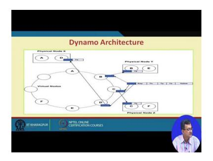
So, this is typical architecture of the Dynamo where there are several virtual nodes and different physical nodes and they are logical connectivity are zone.
