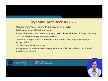
So, if you look at the Dynamo architecture. So, it is a key value pair with arbitrary value key value pair with arbitrary arrays of bytes like it uses MD 5 generates a one twenty eight bit1hash table hash value.
