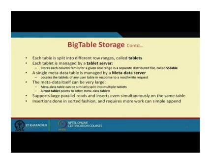
So, a single meta-data table is maintained by the maintained by the many meta-data server the meta-data itself can be very large. So, the meta-data while storing this itself can be very large, in that case; it is again broken down into split into different tablets a root tablet points to the other meta-data tablets.
