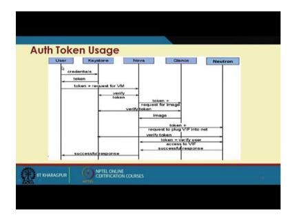
And if we look at the token exchange mechanism; so, the user to the keystone it is; for the identification or authentication, then it goes to the nova, then the glance and the neutron. So, this is what we say; if you look at that process flow of that particular authentication token uses.
