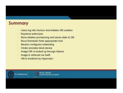
So, in summary if you have a quick overview of the whole this open stack, the user logs in horizon and initiates the VM creation. Keystone authorizes it, nova initiates provisioning and saves state to the database. Nova scheduler finds the appropriate host. Neutron configures the networking aspects, cinder provides block devices. Image URI is looked up through glance.
