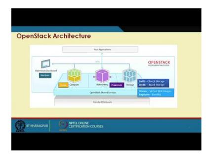
So, if you look at from the point of view; then you have the standard hardware at the backbone, then the open stack shear services and over that we have compute networking
