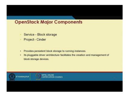
So, another type of storage service is your block storage, which is provided by cinder provide persistent block storage to running instances. So, it is a persistent block storage to the running instances; it is pluggable driver architecture facilitate the creation and management our block storage. So, it is a; again it is a persistent storage and persistent block storage and provides a pluggable driver architecture to facilitate creation and management of block storage things.
