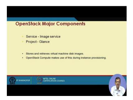
So, the next component is glance or what we say that image services. So, it basically open sack support separate type of images or image services where which can be loaded or which can be instantiated into that different VMs. So, I can have different VM and different images of say operating systems and other things can be instantiated on the difference VMs based on the user needs and requirement.
