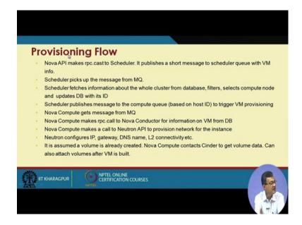
Similarly, there is a provisioning flow nova appearing makes a rpc cast to scheduler; scheduler picks up the message from the message queue, scheduler fetches information about the whole plaster from the databases, data base filters; selects compute nodes
