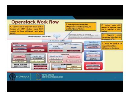
Like, if you look at the open stack workflow; so, these are the different components are there nova for compute, cinder for block storage; these are the compute nodes in the nova. There are other components within the nova, there is a cinder also have its own component. Neutron is the networking part; networking aspects; so, neutron API scheduler plug in, queues etcetera these are all networking related component.
