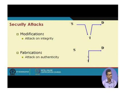
So, this is attack on availability this availability is block this is attack on confidentiality like you are sending from a to b or s to d and somebody else, that intruder I is listening to that it can be attack on modification, that this attack on integrity of that data right; so or even the origin right. Source is sending to d, but in between there is a intruder I which
