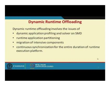
So, if we look at the runtime offloading there are different tricky issues right or factors like a dynamic runtime offloading involves the issues of dynamic application profiling and solver on SMD right runtime application partitioning you need to partition the it is runtime migration of intensive come component like which are computational intensive component need to be migrated.
