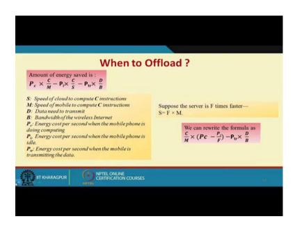
So, if we look at a very straightforward formulation of the things. So, if we look at that equation that. So, what we say that  $P_c$  is the energy cost per second when the mobile phone is doing computing; that means, mobile phone is computing  $P_i$  is that energy cause the mobile phone is idle.
