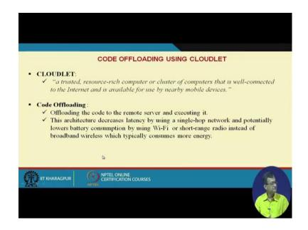
So, there are other trials or other type of a initiative one is that code offloading using cloudlet right. So, if you look at cloudlet, it is a trusted resource rich computer or cluster computers that is well connected to the internet and is available for use by nearby mobile devices. So, it is a what we say we can look at as a smaller version or of cloud, but it is resource rich, but it is more within the locality of the mobile devices or nearby regions right.
