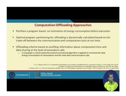
So, party computation overloading there are several approaches, you can see several research papers also partitioning a program based on estimation of energy consumption before execution. So, what we say that pre partition estimation of the thing, optimal program partitioning for offloading is dynamically calculated based on trade off between communication and computational cost at the at run time.
