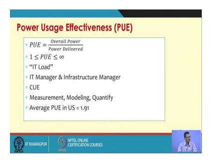
There is some effort of looking at the power usage effectiveness measure to find out that what is PUE and how to measure that how the how effectiveness is this power uses. So, there are different theories behind this. So, this there rough cart measures that how whether we can measure this power usage effectiveness of a typical infrastructure or a typical cloud service provider.
