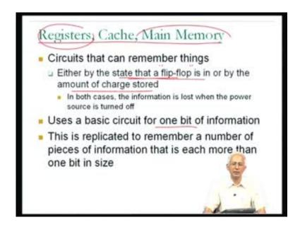
But, what we have seen about the different kinds of memory that I have sub listed in other words, registers, cache, and main memory is that these are all made out of circuits that can remember things. They made out of electrical circuits, digital circuits that are capable of remembering things and the way that the circuits remember is either by the state of a circuit, some of the circuits are known as flip-flops.
