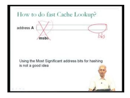
Therefore, using the most significant address bits does not seem like a good idea in the special case of small programs, it would be the case that pretty much everything would index into the same place in the hash table, they would have the same hash function. Therefore, it is not a good idea to use the most significant bits for the fast cache look up.
