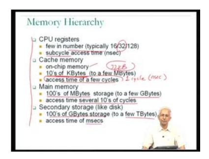
Finally, secondary storage like disk we do know that, I have talked about disks which could have 100s of gigabytes or even a few terabytes of capacity. And that the access time is not on the nanosecond time's scale at all, but in fact, on the millisecond time scale.
