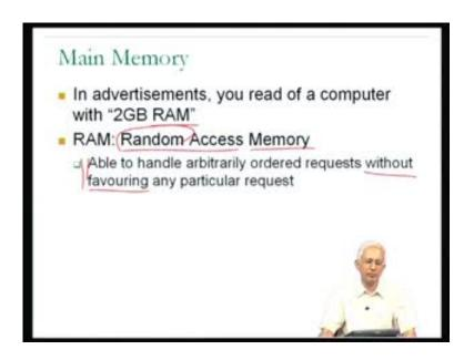
Now, one term which is used in connection with main memory and which I have also use in this class is to talk about RAM, R A M. I used in this every lecture because, when I talked about, when I replaced, when I give you the block diagram of cache and I started by saying cache has fast memory, but then when I went to a technical mode, I replaced the word fast memory by cache RAM, R A M and I never told what R A M was.
