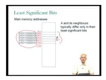
Once, we will look at a picture of the memory image and let us consider a particular... this is the address A that I am concerned about, and I know that address A has some address, but this could be the address I am just putting down some, this is not 32 address it is only a 16 bit address, and in red I have shown you the least significant bits of the address A.
