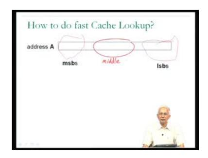
Now, there are a few possibilities, one possibilities is that I could use the most significant bits of the address A and other possibilities that I could use least significant bits of the address A and of course, the third possibility is that I could use some of the intermediate bits of address A.
