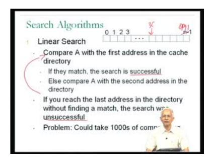
So, this is the size of the problem, a few thousands, in our particular cache example, it was about 8000 based on a current calculation, but remember that our requirement is that this search should have been extremely fast. So, we are trying to understand how search can be done quickly, and the requirement for speed comes from the fact that the entire
