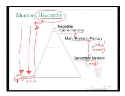
So, there was interplay between main memory and secondary memory from the perspective of virtual memory. We are now talking about cache memory and we realize that what the cache memory is containing in its cache RAM is, some blocks out of the many blocks that are present in the main memory and not all the contents of the main memory can be present in cache memory at a given point in time, given that the cache memory is so much smaller than the main memory.
