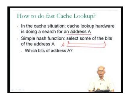
We now understand that in order to do fast cache look up, the cache hardware must be using a hash function. Now, a hash functions on what? In our cache situation, the cache look up hardware is doing a search for an address A and therefore, the hash function must be computed on the address A.
