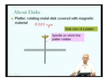
So, this is the platter and it has a magnetic coating on it, which is what I am showing by this yellow color. Now, if I look at it from the side, this once again is the hard disk, the platter looked at from the side. Recall that it is rotating, which means that, it must be rotating around its..., I had showed you the center of the of the disk.
