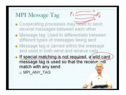
And therefore, MPI actually give us an option for message tag which is what is called a wild card. It is basically wild card indicating that it is not a specific value of message tag, but some general kind of a notation for a value. And this is to be used in the special case where we do not really want to match a particular send and a particular receive, but do not mind which data is received by any one of the receives in process P 1 in our example.
