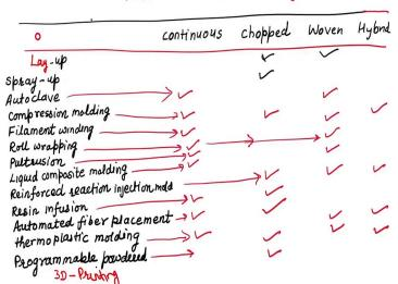
Fabrication Process for Polymer Matrix
