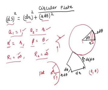
Now, I am going to explain to derive or deduce that set of equations for a circular plate. If you take an example of a circular plate, take a small element at distance r and that distance will be dr and this will be  $d\theta$ . In that case:
