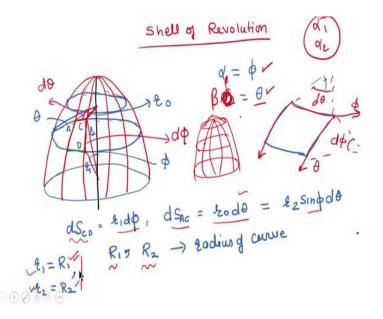
Now, the shell of revolution: this is the most generalized form, we have already classified the shell. The first classification is by the revolution of the surfaces i.e., we can generate the surfaces by translation through a parametric line.
