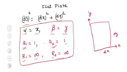
Let us say, we want to find the equation for a flat plate, can we deduce the plate equation from the shell governing equation? For the case of a plate the parameter
