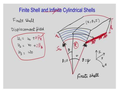
First of all, here a finite shell is considered to study, the displacement field in this paper
