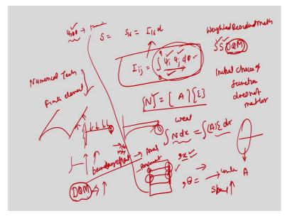
Here the S is the most important part, it is nothing but it contains all the components. Let us say,  $S_{16}$ , there it shows  $I_{16}d$ , where  $I_{ij} = \int_{\theta}^{\alpha} \psi_i \psi_j d\theta$ , if we convert it into a weak form. Initially, we knew  $\psi_j$  along  $\theta$  direction, so we have chosen any function and converted using the concept of weighted residual method.
