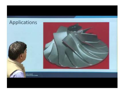
So, the other things like this is also for the complex design of the guide vanes or the blades which can be easily made using the casting process.
