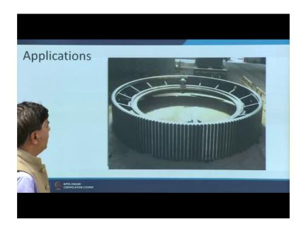
And this is a very large size girth gear which is also made by the casting followed by the machining in order to have the desired geometrical dimensions.
