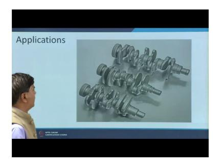
And then further this is the crank shaft which is made through the casting routes and this is subsequently machined and then grinding is carried out in order to have the desired the tolerance as well as the surface finish
