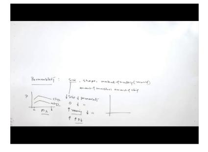
So, considering like permeability; which is about the ability to allow the escaping of the gases, which are present in the mould? So, like size, shape, and the method of moulding; basically it is about the ramming, how the ramming is being done. The amount of moisture amount of clay which has been added;
