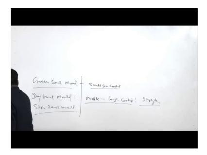
But this is especially good for the small sized castings, where even those somewhat pure strength can also sustain the shape of the mould. In case of the middle to the large size castings large casting it is necessary that a strength is crucial in order to retain the size and shape of the mould. So, for that purpose it is required that whatever mould has been prepared that is properly dried.
