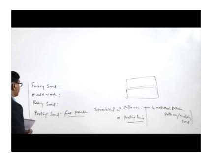
Parting sand is basically this is a very fine powdered sand, which is basically a sprinkled over two things. One is pattern and another is parting line.
