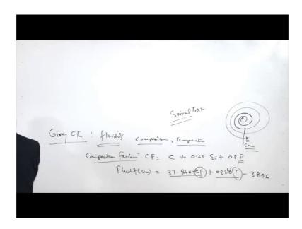
This has very good fluidity under the low melting point that is why it is very easy to develop the castings of the way cast iron and it largely depends upon the composition apart from the temperature. So, composition temperature for the mould of the given for a given mould this what we can say.
