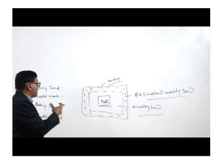
Basically the backing sand is like a; this is the flask. So, and here we have pattern in the top view then the filling of the mould or the flask is achieved through the backing sand.
