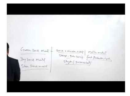
So, among the types of the mould like one is green sand mould, then dry sand mould and then skin sand mould.
