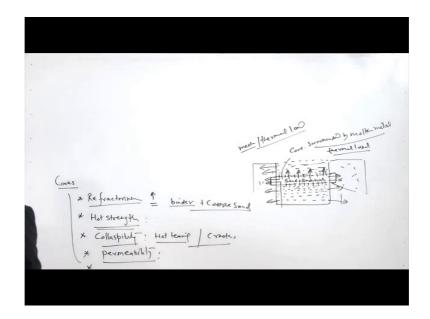
And what these properties are like it should be of the very good refractoriness it. So, refractoriness required in the core is much higher than what is needed for the moulding sand. So, higher refractoriness is needed because it experiences much more thermal loading since it is surrounded by the molten metal.
