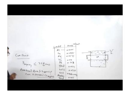
Buoyancy force is less than the 3.5 A in centimeter square then core print area is found to be enough. And if that is not the case then we need to provide the additional area, if this equation is not satisfied then additional area for support of core is provided and for this purpose chaplets are used.
