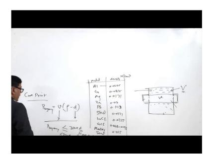
Buy buoyancy force p say will be acting can be determined from the volume of the volume of the core into. So, volume of the core, small v into the density of the molten metal minus density of the sand core, a core sand.
