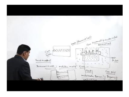
The cores are not used means are not used only with the Sand moulding for producing the internal features of course, the cores are used in the sand moulding, but not only the sand moulding also in permanent moulds cores are used. So that in the permanent moulds means these will be the made of these are the metallic moulds, and in the metallic moulds the core is positioned suitably, so that internal feature and the cavity or the hole can be produced.
