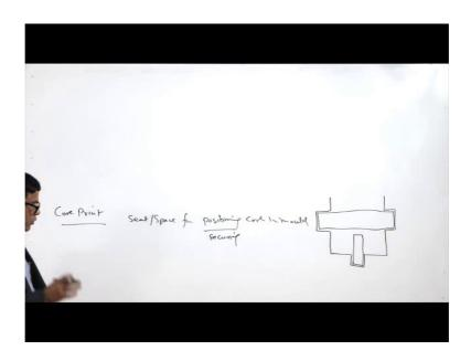
Now we will be talking about the core print. Core print basically it provides the seat or the space. Seat or space for positioning the core in the mould.
