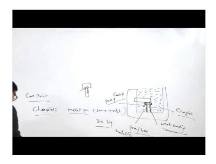
Chaplets these are the metallic pieces most of the time same metal is used for this purpose same as that of the casting. So, if the say this is the mould and the core is positioned in this manner, it is overhanging means the depth of the hole here is partial and this is the core. So, in this case we need to provide support to the core with the help of a chaplets. So, this is the metallic piece which will be used to provide the support to the core.
