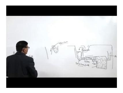
So, it is basically as I have said this is the reservoir of the molten metal which will be receiving the molten metal and it is designed. It can be designed in the 2 ways one is a simple like this. So, here the molten metal is there and then it will be reaching to the sprue. And another design here we put some obstruction so that the molten metal when filled in the pouring basin.
