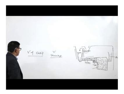
So, say the volume of the casting for that purpose we need to determine and with respect to the volume we need to consider. What is the volumetric shrinkage of the metal on account of the liquid to solid state transformation? And for that purpose what we need to consider is the metal which is being subjected to the casting means which is being processed by the casting rout.
