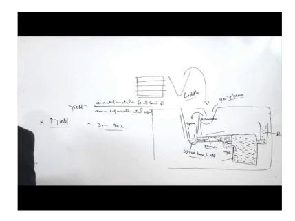
What is the yield basically the amount of the molten metal used divided by, oh sorry amount of the molten metal used a ratio of the amount of the metal in final casting.
