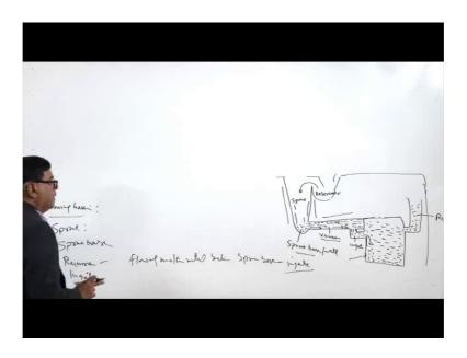
So, basically the runner facilitates the flow of the molten metal between a sprue base and the in gate. It is normally designed this sprue runner is normally made in the cope portion of the mould and that well the drag.
