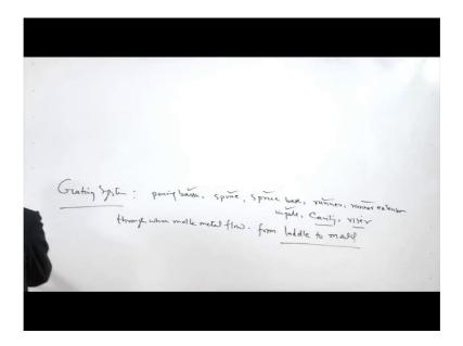
Gating system comprises number of the elements or the parts, which includes like pouring basin. Then like sprue then sprue base, then runner and then sometimes a runner extension is also there. And then in gate after the in gate we have cavity or the mould and then riser. So, these are the different elements through which you see this is the sequence through which molten metal flows from the ladle to the mould.
