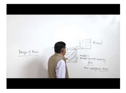
We know that the role of the riser is to feed the molten metal to the mould so that the shrinkage related with the liquid to solid state transformation can be compensated, but to perform this role; say this is the mould and here we have riser. So, if any shrinkage is taking place due to this transformation from the liquid to the solid state, that needs to be compensated by feeding the molten metal present in the riser.
