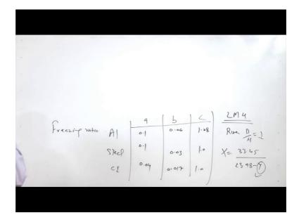
So, like a for aluminium 0.1, for a steel 0.1, and for cast iron 0.04 and b for aluminium is 0.06, 0.03 for a steel and 0.017 for cast iron. Similarly c for aluminium is 1.08, 1 and 1 for cast iron. One typical freezing ratio for one of the commonly used aluminium alloy L M 4 freezing ratio for the riser, when the diameter to the height ratio is one the freezing ratio is given by the equation 33.45 divided by 23.98 minus y.
