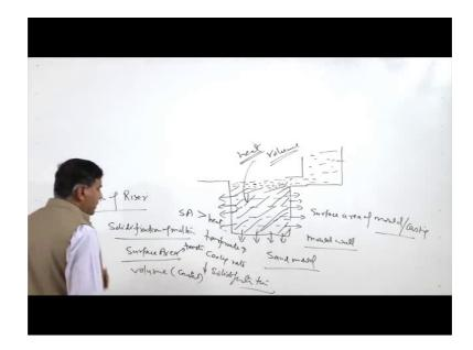
So, this solidification we know that the solidification of molten metal depends upon the fact that, how fast heat is transferred from the molten metal to the mould wall. So, all around we have mould walls. So, if these are of the metal, then they will be extracting heat at much faster rate as compared to the case when they are made of the sand mould; the walls are made of the sand or the moulding sand.
