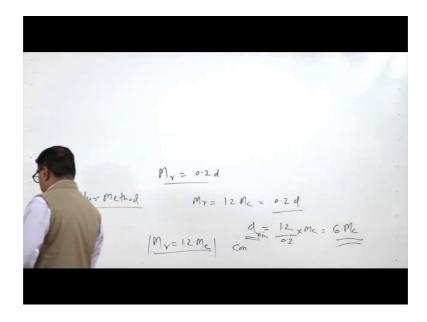
So, in that case since the M r this M r. So, M r is equal to 1.2 times of the modulus of the casting is equal to 0.2 times of the diameter of the riser. So here this is what we can say that in the diameter of the riser will be equal to 1.2 divided by 0.2 into the M c. So, it is basically the 6 times of the modulus of the casting. This is how we can determine the diameter of the riser and because assuming that the diameter.
