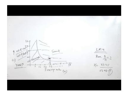
So, freezing ratios from 1 to say 1.9 the interval of say 0.1 we can say. So, 1, 1.1, 1.2, 1.3 and likewise to 1.9 and here the volume of the riser to the volume of the casting this is basically the value of the y in our equation. So, the relationship between basically the x and the y and what it shows.
