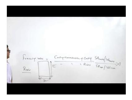
So, in case of the cylindrical shape rises basically the length and the diameter of the riser is obtained as for as the design is concerned. So, basically efforts are made to determine the diameter to the diameter and the length of the risers. So, that the desired freezing ratio can be achieved so, here some freezing ratios for the cylindrical shapes have been equations have been developed for operating.
