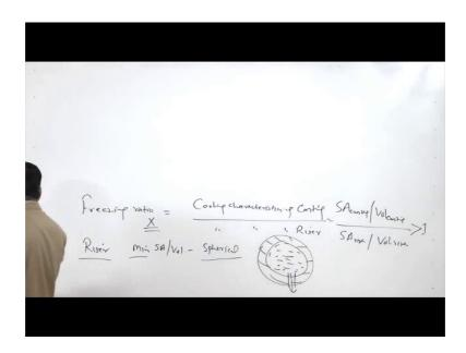
Also has been obtained or developed which is basically the ratio of the cooling characteristics of the casting to that cooling characteristics of the riser.
