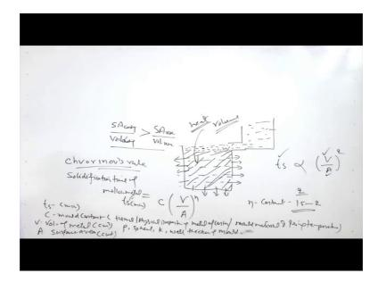
Solidification time of the molten metal it can be say in casting or in the riser this can be given with the help of like say t c in t s in minutes means the solidification time in minutes.
