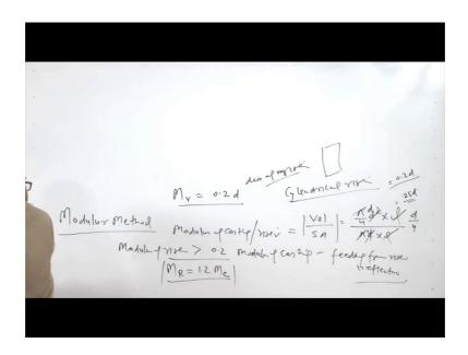
The Modulus is the inverse of the cooling characteristics means cooling characteristics we have determined cooling characteristics we have determine we have defined as a ratio of the surface area to the volume. So, the modulus is the inverse of the cooling characteristics means modulus of the casting or the modulus of the riser will be the volume to the surface area.
