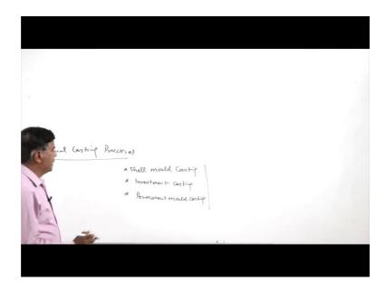
There are three casting processes a special casting process about which we will be talking about one is like shell mould casting process, then investment casting process and then permanent mould casting process. So, in this presentation basically I will be focusing in the shell mould casting process.
