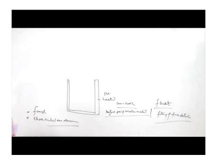
So shell is like this. So, this shell which is been produced is basically heated or what we can say it is pre heated pre heated. This pre heating can be done in the range of 100 to 1000 degree centigrade before pouring the molten metal.
