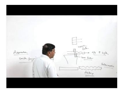
So, hammer is used to beat the metal. So, that desired manipulation is achieved. So, one typical the process which is called fullering in black forging a sorry smith forging process a wherein over the anvil say this is the anvil having the hole in which the fuller is placed like this over the anvil and so this is the lower fuller and over this like this. So,
