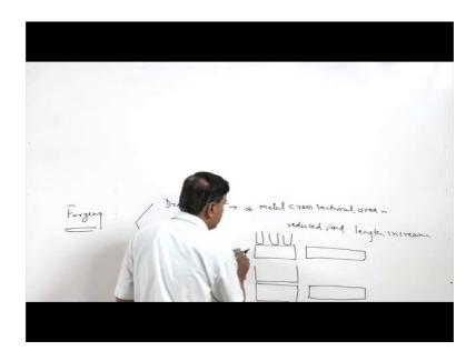
So, in the forging whenever there is a plastic flow of the metal depending upon the way by which thus desired shape is being achieved by the application of the force we say it the drawing out or the upsetting force; these are the 2 broad categories, in case of the drawing out process of the forging basically the metal cross sectional area is reduced and or the length increases. So, basically the job along it is in a; during the drawing process and so here like the job is like this.
