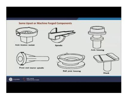
So, these are the different products which can be made having the one end of the smaller cross sectional area, then the other end and these kind of the shapes can be made easily using the machine forging process.
