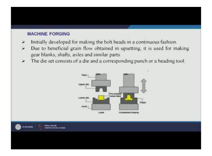
So, as far as machine folding just as I have described; the initially the machine forging has been developed for making the head of the bolts in continuous fashions and advantage of this, it helps to regulate the flow of the grains in such a way that we can
