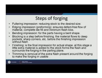
So, if we see here, yeah, these are the steps of the forging like fullering edging bending blocking and the finishing and finally, the trimming.
