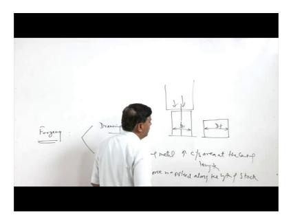
So, here it compresses and reduces the thickness and thereby increases the length while in case of the upsetting just reverse happens and in case of the upsetting the flow of the metal or the plastic deformation increases the cross sectional area at the cost of length basically length reduces and increase in cross sectional area takes place and another thing the force is applied along the length of the a stock or the job.
