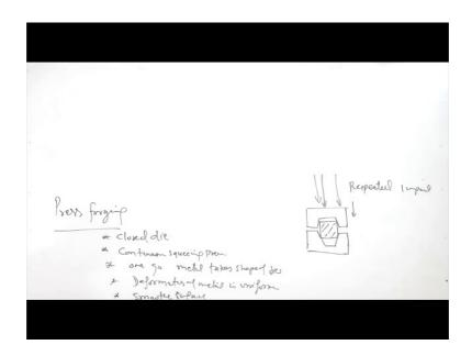
So, here in this case; the important features like closed dies are used uses closed dies and continuous squeezing pressure is used and when the continuous pressure is used in one go in one go the metal takes the shape of the dies on closer and during the squeezing action the deformation of the metal deformation of the metal is uniform through the thickness or throughout the depth.
