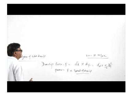
So, if we see the drawing force is obtained using the simple equation, drawing force is obtained force f is obtained from the drawing stress multiplied by the final cross sectional area and we know that final cross sectional area sigma D multiplied by pi by 4 the D f that is the final cross section, final diameter. So, this is how we can determine the drawing force and to determine the power basically, to determine the power consumed in the drawing process.
