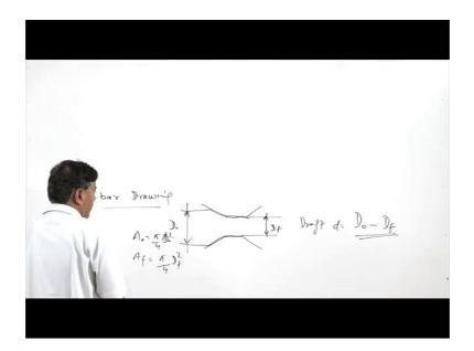
With the change in cross section is the draft, which is draft D, is obtained from the difference in the initial diameter to the final diameter.
