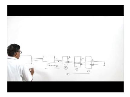
So, for example, here is the mechanical arrangement, which will be used for pulling the carriage, is this one which will be holding the wire, which is being drawn and then here, we will have the die. This is lubrication arrangement, another die, another lubrication arrangement like this. So, basically the wire, which is to be drawn is inserted from here and then it is first lubricated, then it is
