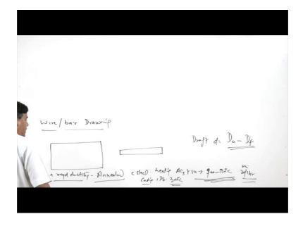
So, what we need the first step is to ensure that is to ensure required ductility. So, for this purpose, it may be required that the metal is annealed properly; so depending upon the kind of metal systems annealing. Say, for the carbon steels annealing are carried out by heating the bar above the AC 3 temperature plus 50 degree.
