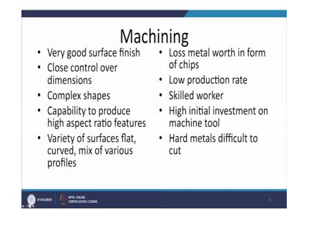
So, the advantage side very good surface finish very close control over the dimensions, and very complex shapes can be produced. And its capable to produce very high aspect ratio features which otherwise cannot be made using the like forming and the casting processes, and the variety of surface features like the flat curved or mixed of the various profiles can be easily made.
