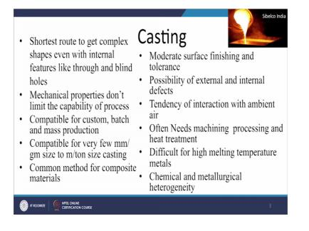
A another important thing mechanical properties of the material do not affect the success of this process the more, because whether it is material is hard or tough or very strong or very low ductility or of very high ductility, that does not affect the processing capability of the casting to get the desired size and shape. So, mechanical properties do not affect or do not limit the capability of this process, and compatible for custom batch and mass productions.
