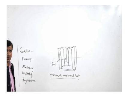
We find that the pure metal solidify solidifies first, and gracefully the impurities or the alloying elements will be segregating or will be moving towards the center, and at the end what we find that all the impurities have got segregated at the center.
