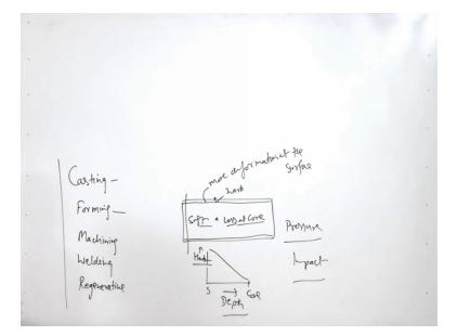
I will explain little bit more the anisotropic e x structure and the properties of the form component we know that in the deformation, we apply either we apply pressure for causing the deformation or we apply impact. So, in case of the pressure and in case of the impact, in case of the impact the deformation is not uniform throughout the section like the surface layers will be deforming more as compared to the inner core material.
