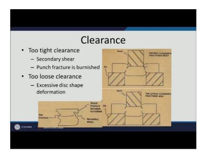
So, here when the clearance is the optimum, then what we get and when the clearance is improper then what we get.
