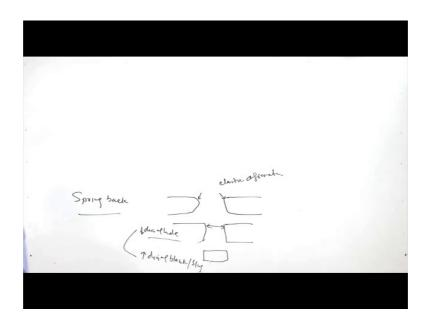
So, if we see the geometry of the whole it this is the kind of the whole edge which is produced. So, this portion actually remains under the elastic deformation in course of the shearing. So, when the punch goes off this portion gets straightened like this and because of this kind of the straightening the whole diameter gets reduced. Similarly in case of the slug straightening leads to the increase in diameter of the slug.
