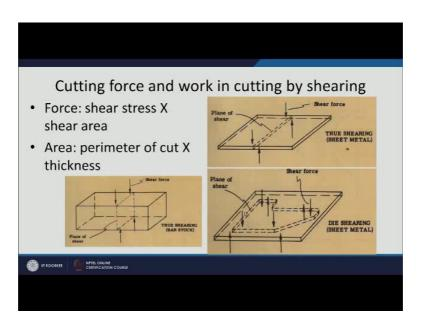
So, Shear force is obtained through the shear area and the shear strength shear again shear strengths are used to determine the force required for shearing basically, it uses the shear area is obtained through this; this is the plane of the shear and which is obtained through Shear force is Shear force multiplied by the shear area; shear area is basically parameter of the cut in to the sheet metal thickness. So, this is the parameter of the cut multiplied by the sheet thickness.
