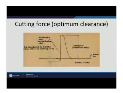
This is the diagram which shows the kind of the cutting force variation in course of the shearing when the clearance is optimum then what we can see these increase in force is very clear and it is vertical and then there is no. This is the case, when there is no secondary shear. So, this is how the force varies in case of the shearing when the
