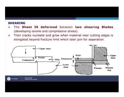
So, we will go through the slide some of the slides first regarding the effect of the clearance. So, this is what I have already said that in the shearing; we used one die and punch; there is a upper blade and the lower blade when the punch move is down the strain is generated into the sheet metal and when it crosses the cracks nucleate; both the sides here and then their propagation leads to the shearing and the separation of the material.
