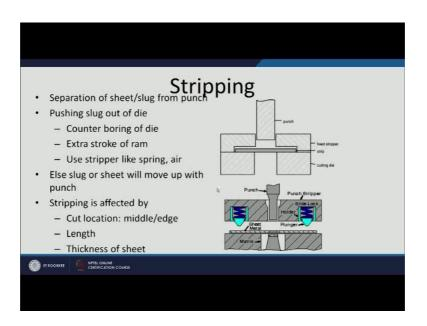
So, the whole diameter due to the spring back effect gets reduced while the diameter of the blank is increased Stripping is needed primarily for the separation of the punch from the die. So, that it can easily be cleared.
