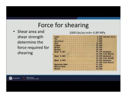
We know that the shear strength of the different metals is well established. So, this is what we can see shear strength 2 different metals like for lead it is in 3500 Lbs per square inch of for aluminum it is eight thousand lbs per square inch and this can be converted in the MPa. And so likewise for the different metals the different shear strength are there and which can be used for calculating the Shear force.
