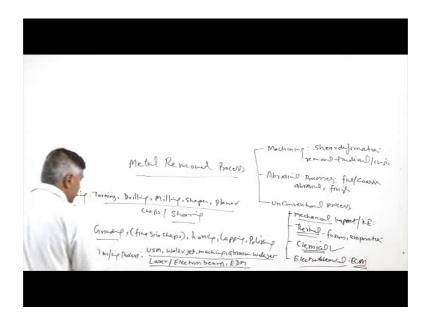
So, under the family of the material removal processes, there are three broad processes category of the processes these are like, machining, abrasive based processes where abrasive material is used abrasive processes and unconventional processes these are also termed as nontraditional processes.
