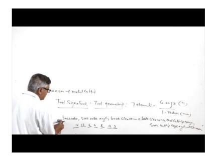
Tool signature indicates or shows the tool geometry of single point tool, where in the different angles as the nose radius are written in a specific sequence.
