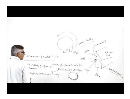
So, if we see here like say this is the tool and this is the clearance so, better to understand first about the tool before getting into the mechanism like say the cutting. So, we will try to see first the single point cutting tool. There can be single point cutting tool or multi point cutting tool. Single point cutting tool basically involves the one cutting edge.
