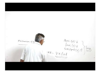
Similarly, feed f is selected very low and the cutting speed is selected high for the finishing operations.
