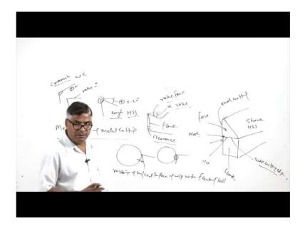
So, the to avoid the basically rubbing of the machined surface of the work piece with the flank of the tool, some inclination is given if we do not give this kind of inclination then you will see this portion of the flank will be rubbing with the machine surface of the work piece. And so, that is how it will be adversely affecting the surface finish of the machine work piece.
