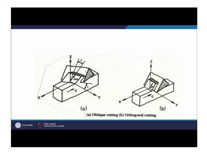
This is the same the figure here where this is the tool and this is the cutting edge cutting edge is inclined, with respect to the velocity direction. So, this is the case of the oblique cutting wherein the forces will be acting in the 3 direction, that these are the x direction y direction and the z direction.
