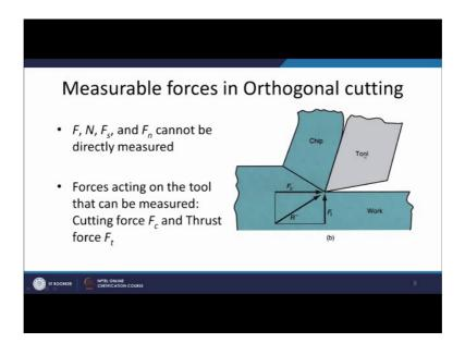
If we move further like say this is the condition that the chip, work piece, the tool, shear plane and the cutting force acting in this direction, and the thrust force is acting in this direction and resultant of these 2 will also be R dash. These are these 2 are the measurable forces which can be measured with the help of the cutting tool dynamometer.
