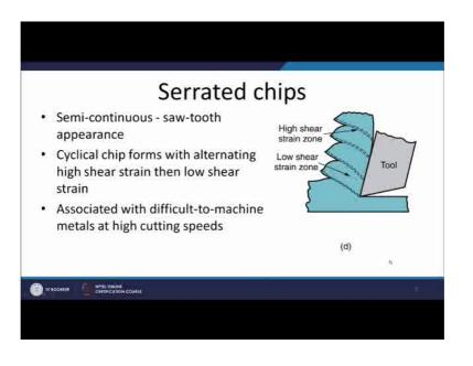
The 4th type of the chip is the serrated chip or segmented chip. This kind of the chip offers typically saw toothed feature. Saw toothed means like if we see any hexa it will have the built blades like this, and which will be performing the cutting.
