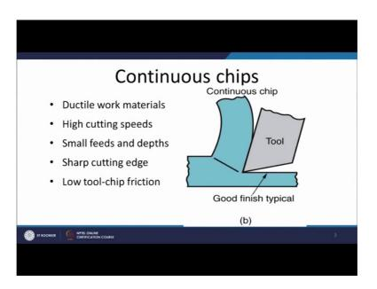
And the conditions under which these are formed, then we will see the built up continuous chips with the built up edge.
