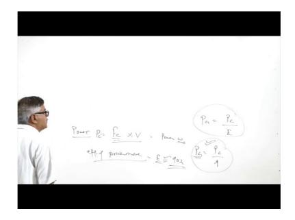
So, the power for machining can be obtained from the F c that is the cutting force multiplied by the cutting velocity. So, if F c is in Newton, and cutting velocity in meter per second, then it will be giving us directly the power required in watt. So, this is one thing like the cutting force multiplied by the cutting velocity will give us the power required for the metal cutting, considering the efficiency of the prime mover or the driver prime mover or the driving system.
