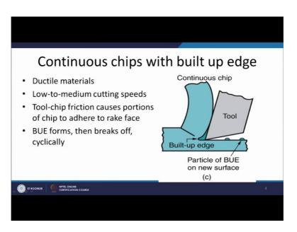
And this built up edge grows gradually and eventually it gets broken, than and when it breaks it is transferred to the chip as well as to the work piece. So, when the built up edge is transferred to the work piece, it adversely effects the surface roughness. Mostly it is a this kind of the chips are formed when the material is soft, ductile and unfavourable cutting conditions. Exist like low cutting speed high feed and depth of cut.
