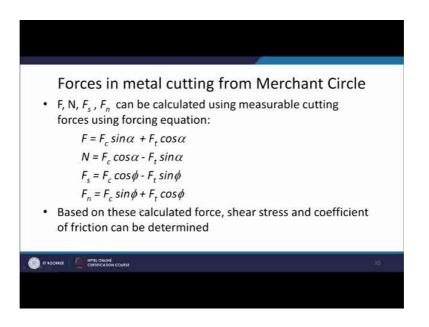
So, the facts force is acting on the tool which can be measured or F c and F t, and these 2 forces can be used for calculating the further other forces like F s, F n, F and n. So, like the friction force F can be obtain can be obtained using the equation, like F c sin alpha plus F t cos alpha. And the normal force can be obtained through the F c cos alpha minus F t sin alpha. These equations are derived through the merchant circle since it requires very elaborate the diagram.
