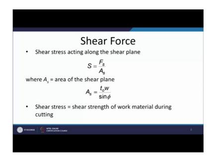
This will give us the shear area. So, this shear area is shear stress can be calculated from the shear force divided by the shear area.
