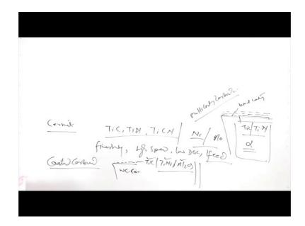
So, for the cermets basically TiC TiN titanium carbide, titanium nitride and titanium carbon I tried are the commonly used by cermets now for making the tool materials and these are, these materials in the powder form are mixed with either cobalt as a matrix or nickel as a matrix sorry the nickel as a matrix or the molybdenum as a matrix. So, these are the reinforcing agents and the matrix is either of the nickel or of the cobalt.
