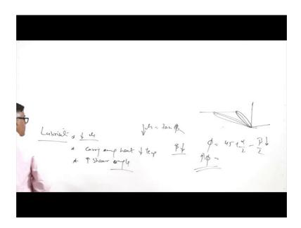
So, when the lubricants are used what we basically get lubricants will be able to reduce the friction between the tool and chip and tool and work piece is one and the second is because of the specific heat and thermal conductivity they will also be able to carry away the some amount of heat, carry away heat from the cutting zone. So, that will be helping in lowering the temperature of the tool as well as work piece.
