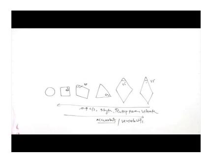
So, this included angle is 80 degree, this angle is 90 degree and then another insert is having the included angle 60 degree, then we may have at 55 degree, like this 55 degree or even 35 degree like this.
