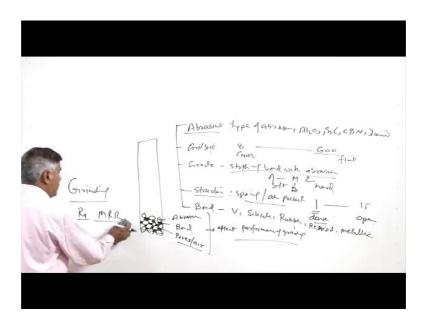
So, the characteristics that we need to see are like this, like the abrasives bonded or held firmly in the wheel. So, these are bonded by the bonding material like this. So, all these abrasives will be bonded by the bonding material in this way. So, what we will see here, there are 3 constituents in that way the one is the abrasive, second is bond and third is some spaces left between the abrasives and bond which we can say as pores where mainly the air is filled.
