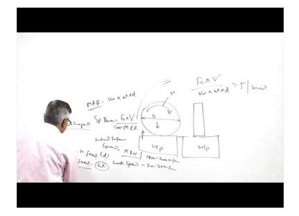
Say this is the grinding wheel rotating at certain speed and in the side view if we see the wheel is like this and it is working on to the surface of the work piece like this is the work piece and this is the work piece.
